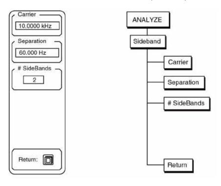
Sidebands are identified according to the formula Sideband  $n = Carrier \pm n$ •Separation where n varies from 1 to the # of sidebands.
