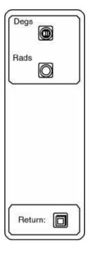
When Phase is being displayed on the active trace, the Units menu appears as shown to the left. Phase values are always between -180 and +180 degrees. The analyzer does not "unwrap" phase.
