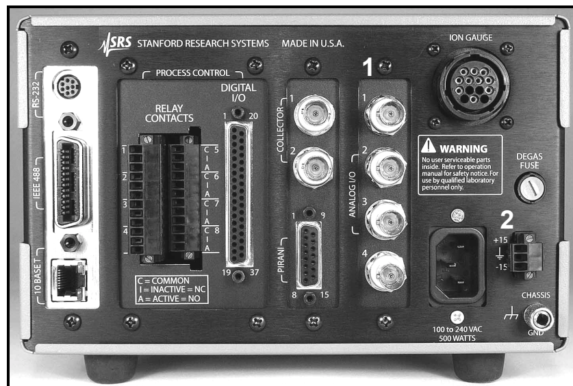
Figure 1-26. Capacitance Manometer Connection Ports. 1. Signal - Four ANALOG I/O BNC Ports. 2. Power - 3-position, terminal block.
