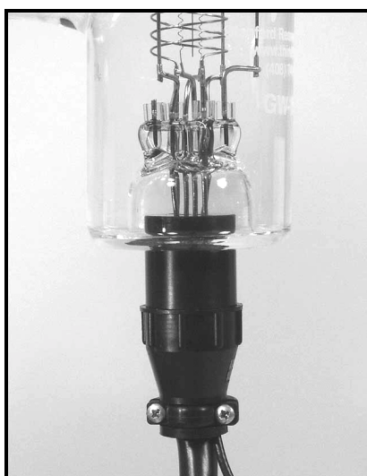
Figure 1-14. O100C2 6-pin connector properly attached to the base of the glass-tubulated gauge.
