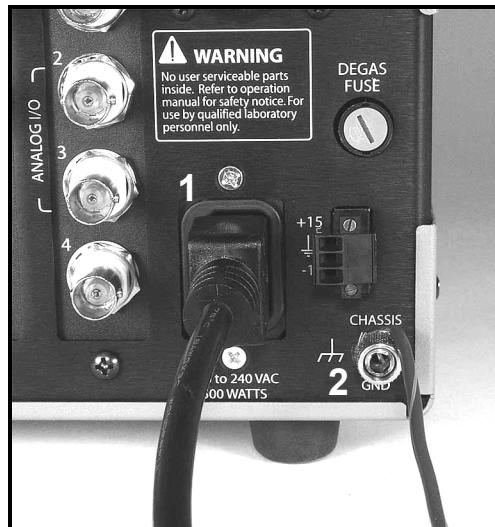
Figure 1-2. Power and chassis-ground connection on the back of the IGC100 controller. 1. Power entry module with power cord (connected to grounded wall outlet on the other end), 2. CHASSIS GND lug with heavy gauge ground wire connected directly to facility earth ground.
