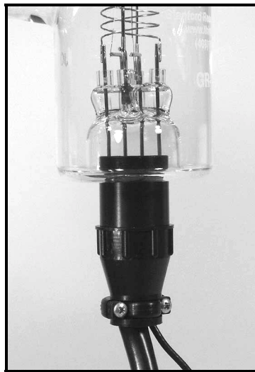
Figure 1-9. O100C1 4-pin connector safely attached to the base of the glass-tubulated gauge.
