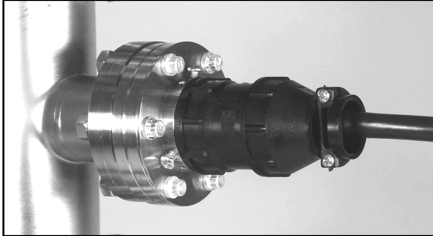
Figure 1-20. Cable connection to the base of a nude ionization gauge with connector shield in place.
