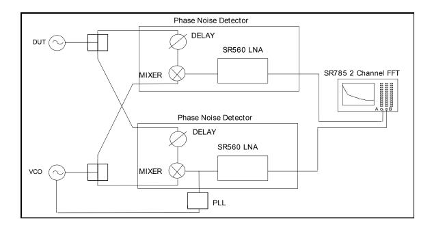
The output of each mixer is low pass filtered and amplified. The signals are then fed into the cross-correlation FFT analyzer. The random noise of the test setup is uncorrelated while the correlated noise is the actual noise of the input signals along with some leakage due to the power splitters.
