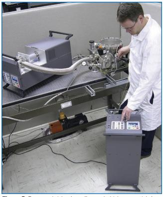
**Figure 3.** Two sample inlets (a capillary and a high vacuum inlet) are shown. And the operating orientations of the UGA, horizontal and vertical, are demonstrated.
