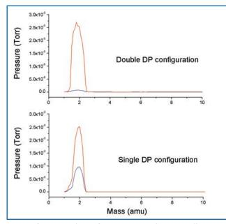
**Figure 2.** Results of the H2 measurements from two different configurations; Single DP and Double DP. The red traces indicate the detector response with the sample valve open, while the blue traces show the response with the valve closed.
