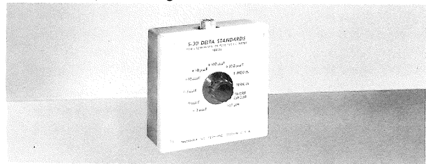
S30 Delta Standards, for calibration of the Type 130 L,C Meter. The unit provides accurately adjusted steps of capacitance and inductance, selected by a rotary selector switch. Values of the capacitance steps correspond to the full-scale adjustments required on the five scales of the Type 130. Two resistors of identical manufacture and similar capacitance, values of 1 megohm and 0.1 megohm, are provided for the resistance compensation adjustment. A 300- \mu h standard permits proper adjustments of the inductance ranges . . . . . $22.00
