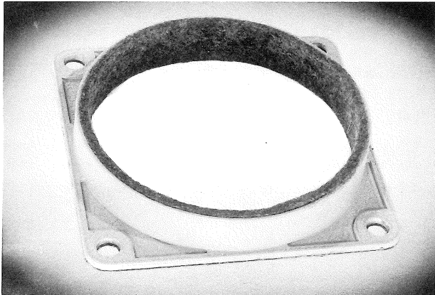
BE510 Bezel, for mounting camera on Tektronix 5" Oscilloscopes. Dimensions—5 7 / 8 " square; ring 7 / 8 " deep, diameter 5 5 / 8 " outside, 5 1 / 8 " inside. Die-cast construction, gray wrinkle finish, felt lined. . . . $4.50
