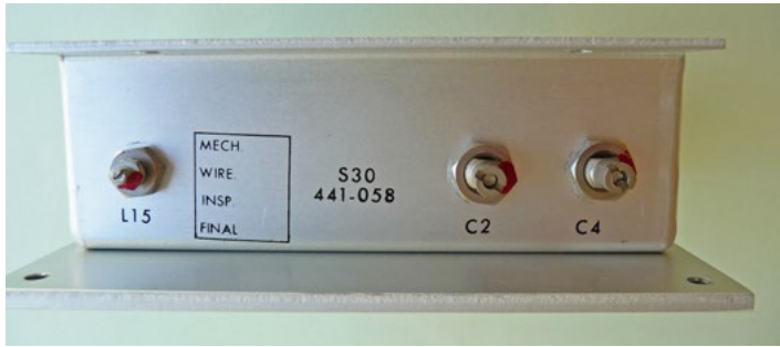
The capacitance and inductance trimmers are mounted on the sides of the S-30 chassis. They are meant to be adjusted as required with the aid of an RLC bridge, and can be accessed by removing the blue case.
