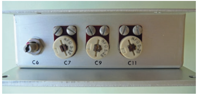
The capacitance and inductance trimmers are mounted on the sides of the S-30 chassis. They are meant to be adjusted as required with the aid of an RLC bridge, and can be accessed by removing the blue case.
