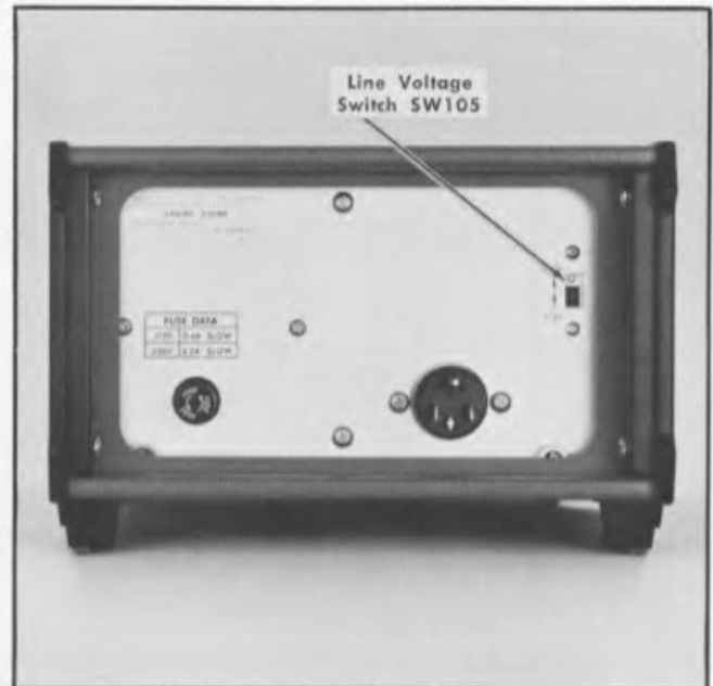
Fig. 2-1. Location of Line Voltage Switch (SW105) on rear panel.
