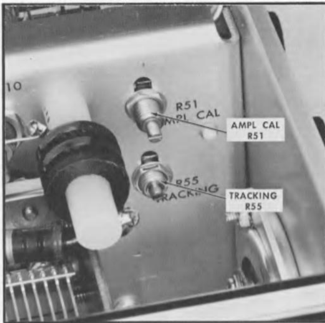
Fig. 6-12. Location of TRACKING and AMPL CAL controls.
