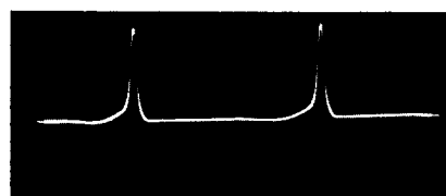
Fig. 28. The same pulse, amplified, at V2 plate. Amplitude 5 volts.
