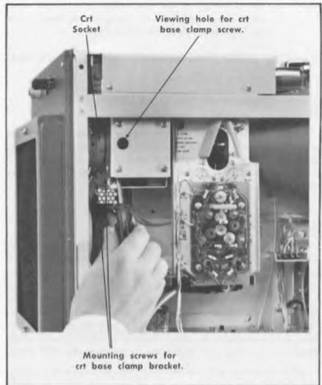
Fig. 4-3. Loosening the crt base clamp.
