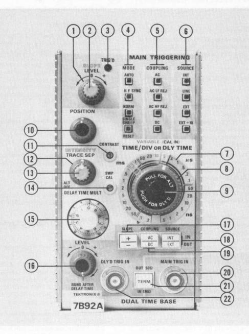
Fig. 2-3. Front-panel controls and connectors.
