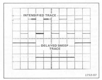
Fig. 2-6. Typical alternate sweep display.
