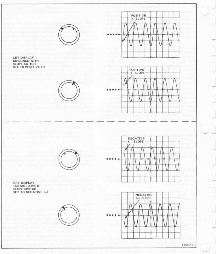
Fig. 2-4. Effect of LEVEL control and SLOPE switch on crt display.
