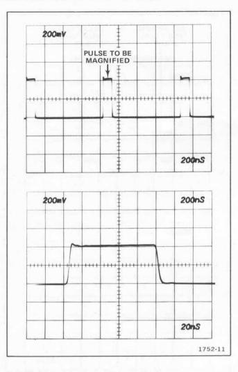
Fig. 2-10. Using delayed sweep for magnification.
