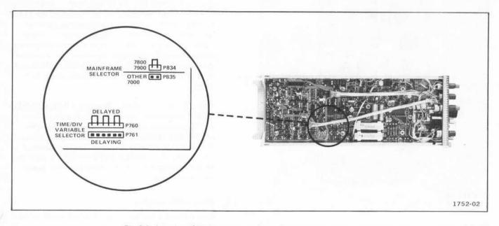
Fig. 2-1. Location of Variable and Mainframe Selector multi-pin connectors.
