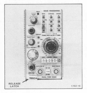
Fig. 2-2. Location of release latch.
