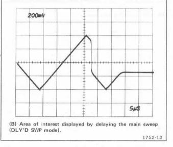
Fig. 2-11. Displaying a complex signal using delayed sweep.
