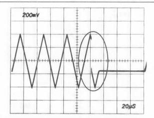
(A) This portion of display cannot be viewed adequately because the main sweep is triggered on larger amplitude signals at the start of the display.
