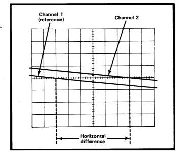
Fig. 2-5. High resolution phase measurement using sweep magnifier.
