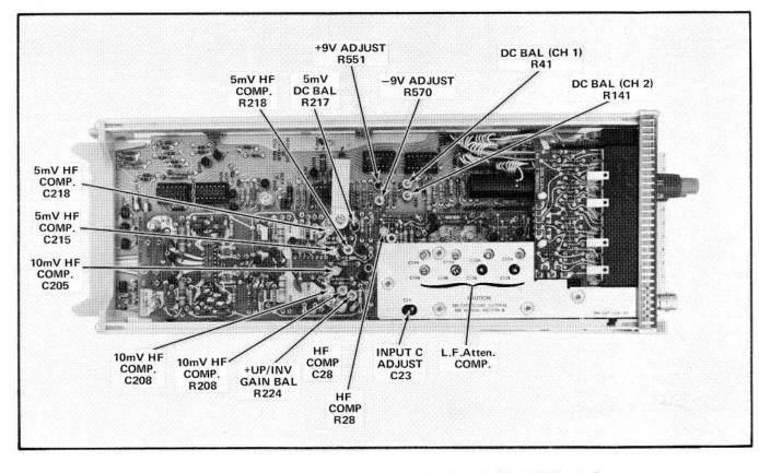
Fig. 5-1. Location of adjustments and test points for Ch 1 side (Ch 2 side identical).
