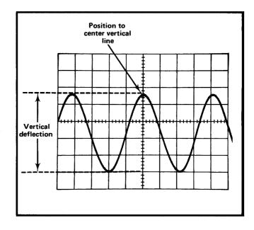
Fig. 2-2. Measuring the Peak-to-Peak Voltage of a waveform.
