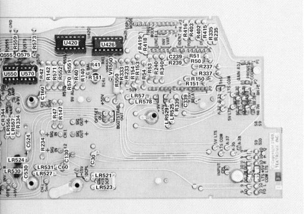
e circuit board showing location of components.
