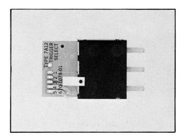
Fig. 7-10. Trigger Source switch and circuit board.
