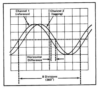
Fig. 2-4. Measuring phase difference between two signals.
