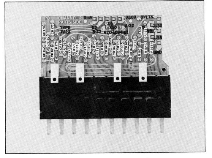
Fig. 7-4, Channel 2 Volts/Div switch and circuit board showing location of components.
