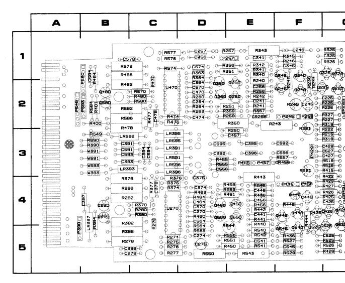
Fig. 8-1. Amplifier Circuit Board Assembly.
