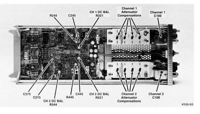
Fig. 4-1. Locations of adjustments used in this procedure.
