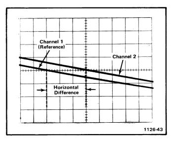
Fig. 2-5. High resolution phase measurement using time-base magnifier.
