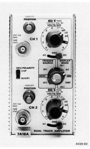
Fig. 2-1. Front-panel controls and connectors. (7A18A shown.)
