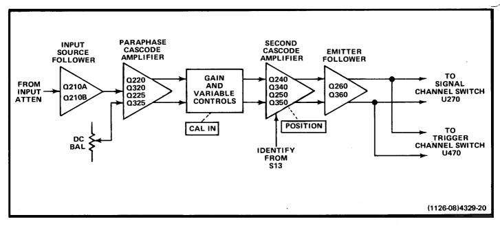
Fig. 3-1. Channel 1 Input Amplifier detailed block diagram.
