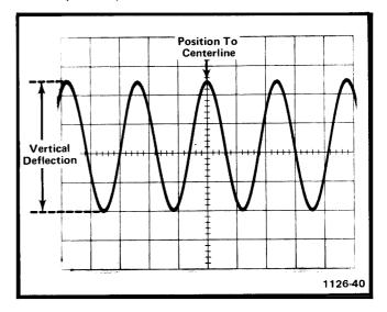
Fig. 2-2. Measuring the peak-to-peak voltage of a waveform.
