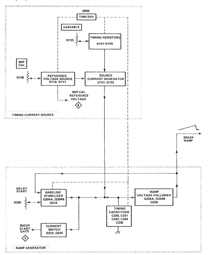
Fig. 3-7. Detailed block diagram of Sweep Generator.
