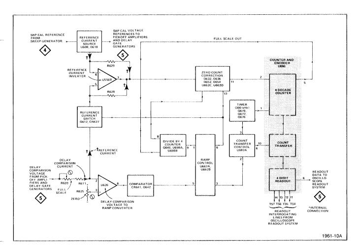
Fig. 3-9. Digital Voltmeter detailed block diagram (SN B088749 & below).
