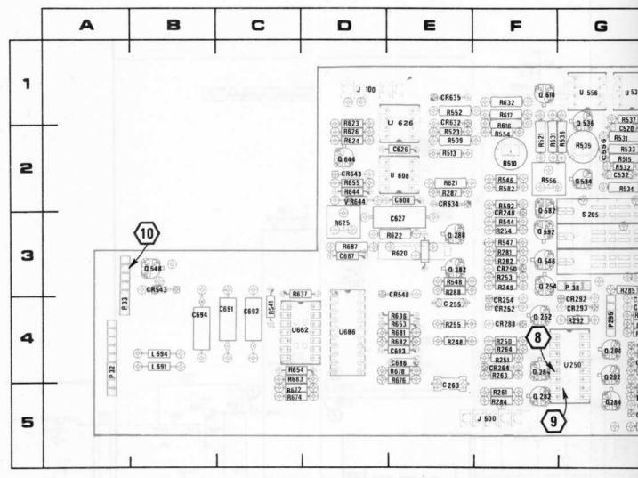
Fig. 8-9A. A4-(SN B088750 & Up) Digital Voltmeter circuit board assembly.
