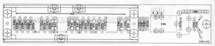
Fig. 8-5. A3-Readout circuit board assembly.
