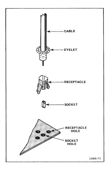
Fig. 4-8. Coaxial end-lead connector assembly.
