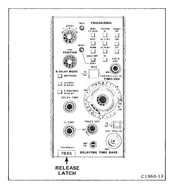
Fig. 1-1. Location of release latch.
