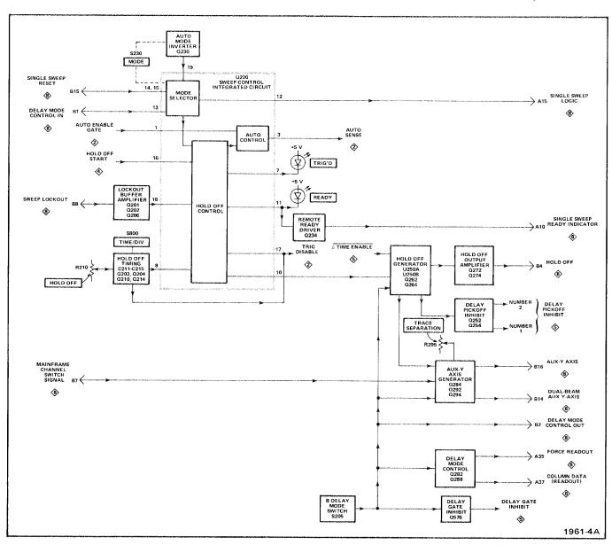
Fig. 3-5. Detailed block diagram of Logic circuit.
