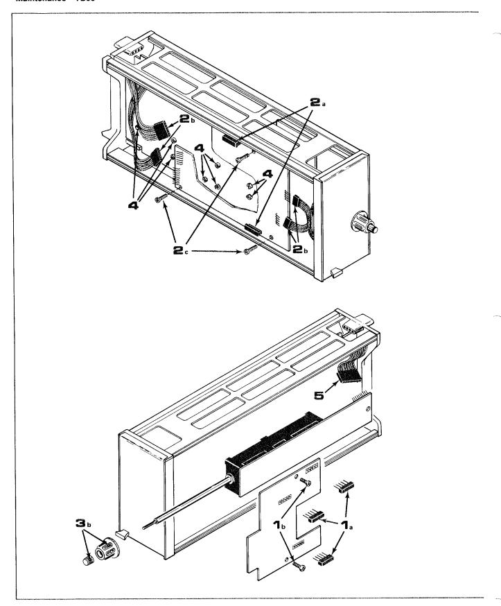
Fig. 4-9. Cam switch removal procedure.
