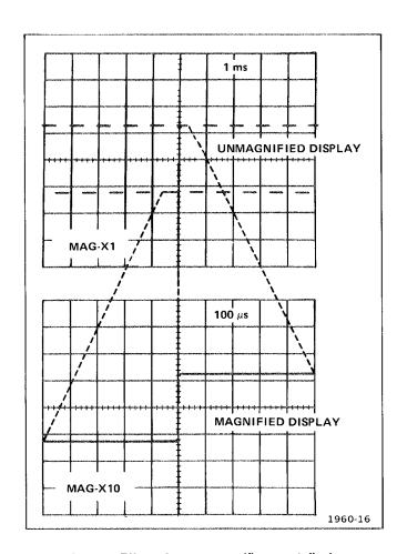
Fig. 1-5. Effect of sweep magnifier on crt display.
