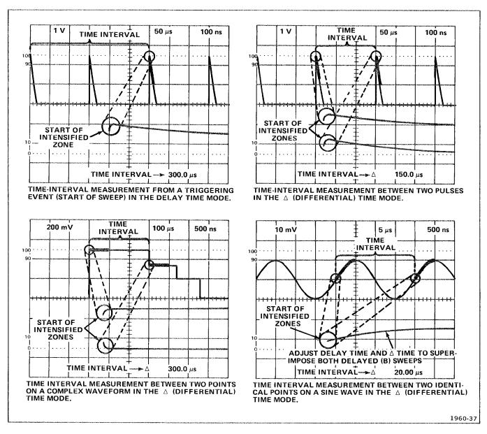
Fig. 1-11. Time-interval measurments in the delay-time and  $\Delta$  (differential) time mode with mainframe alternate or chopped operation.
