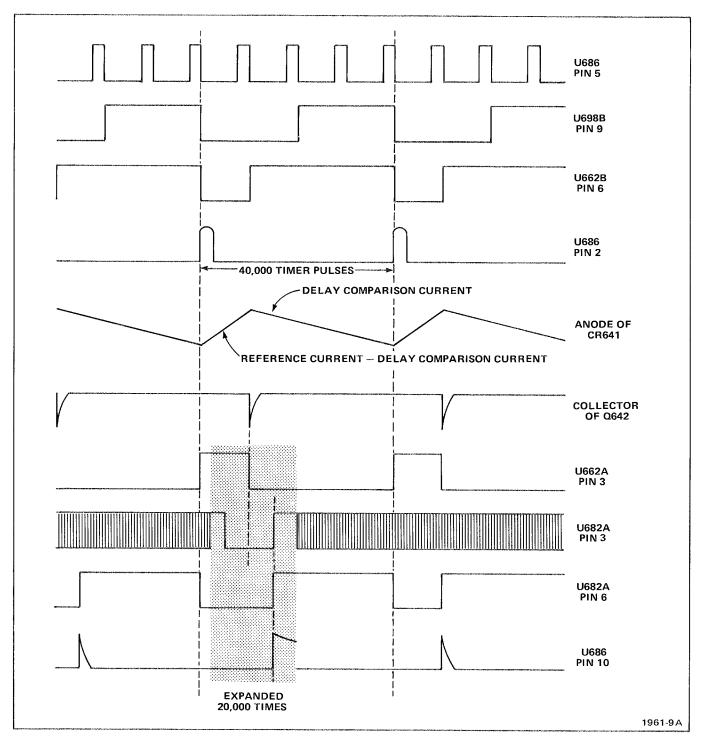
Fig. 3-10. Digital Voltmeter timing diagram.
