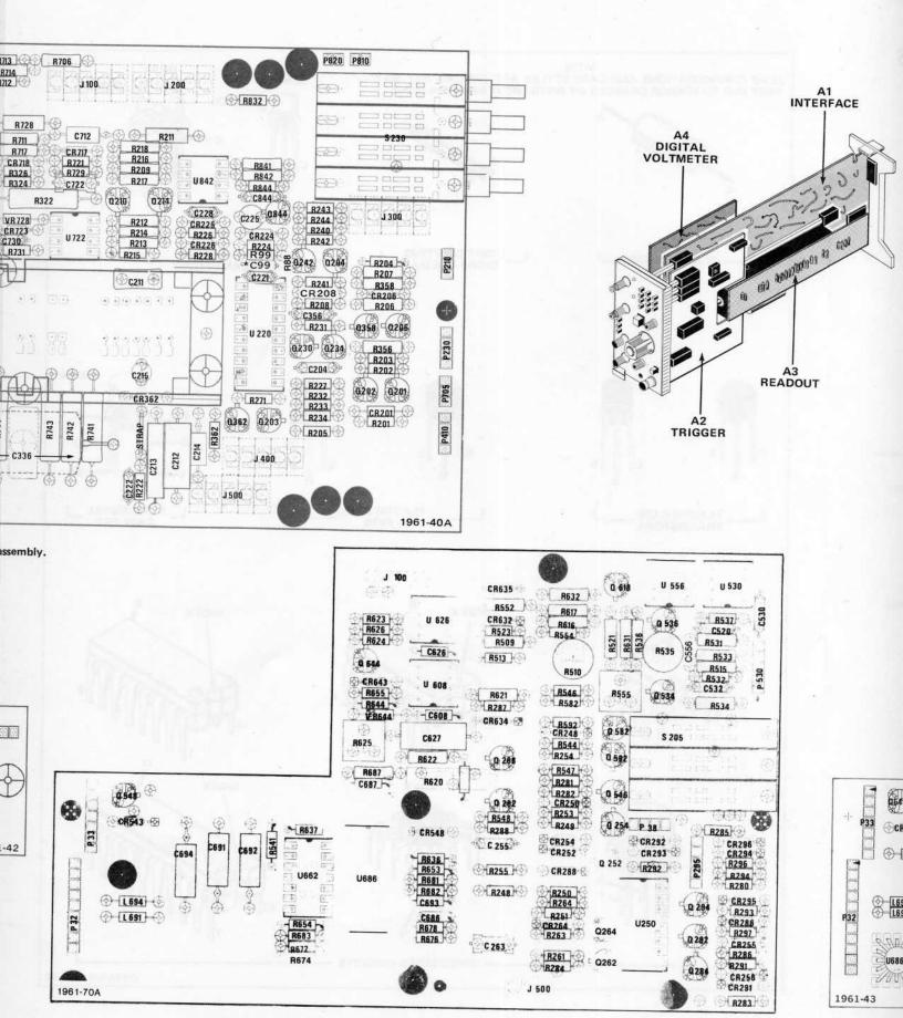
Fig. 8-6A. A4-(SN B088750 & Up) Digital Voltmeter circuit board assembly.
