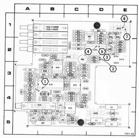
Fig. 8-8. A2-Trigger circuit board assembly.
