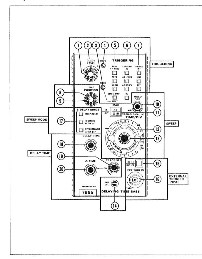
Fig. 1-2. Front-panel controls, connectors, and indicators.
