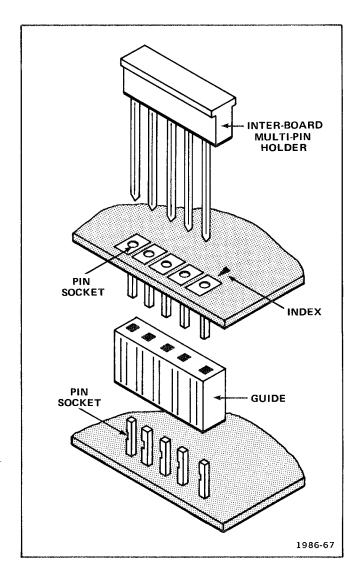
Fig. 4-3. Inter-board multi-pin connector assembly.
