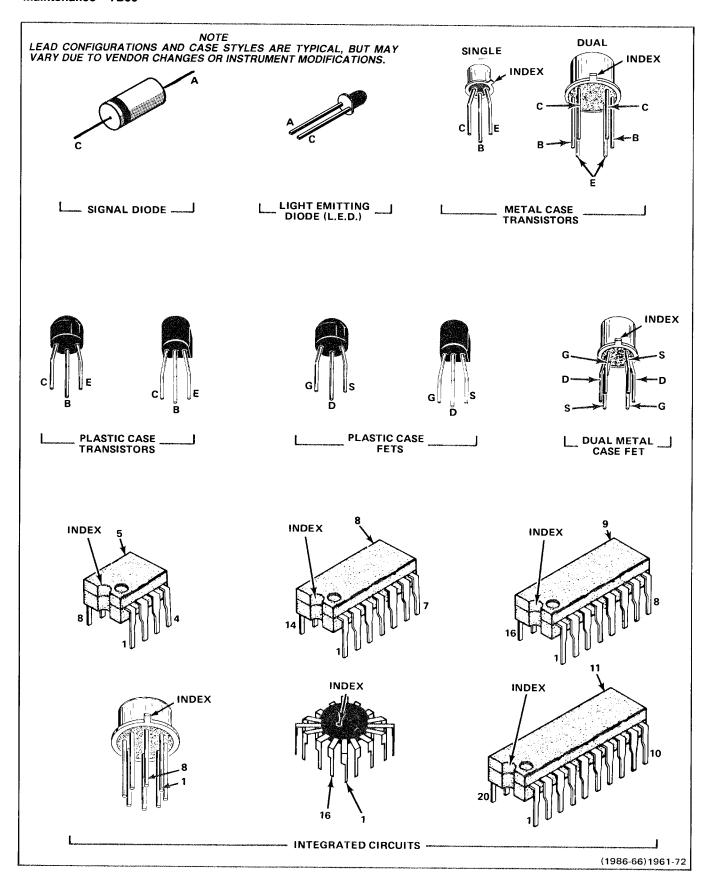
Fig. 4-2. Semiconductor lead configuration.
