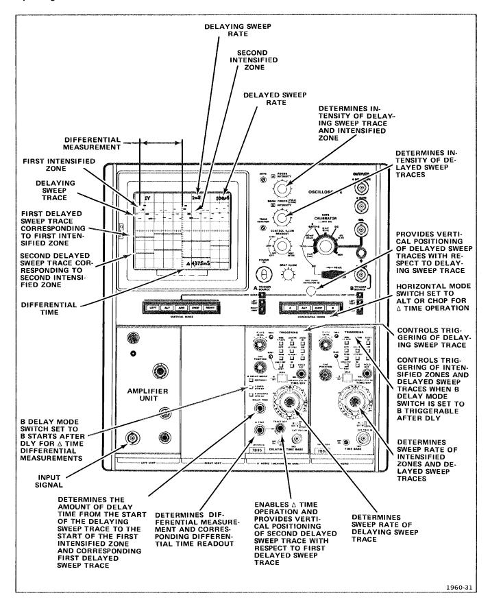
Fig. 1-7. Typical  $\Delta$  (differential) time operation.
