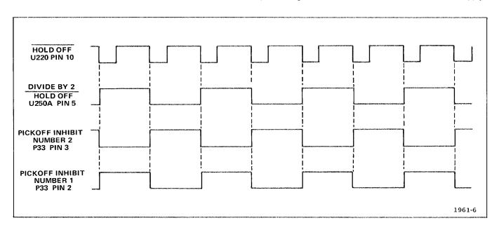
Fig. 3-6. Timing diagram for Delay Pckoff Inhibit stage.
