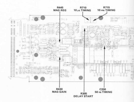
Fig. 8-11. Location of Sweep Timing adjustments.
