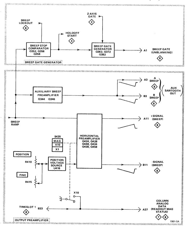
Fig. 3-7. Detailed block diagram of Sweep Generator (cont.).
