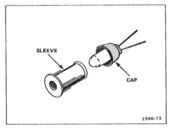
Fig. 4-12. Front-panel light socket assembly.
