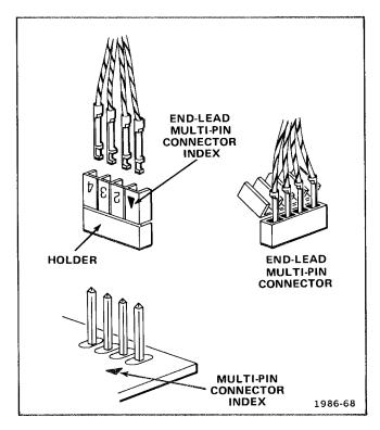
Fig. 4-4. End-lead multi-pin connector assembly.
