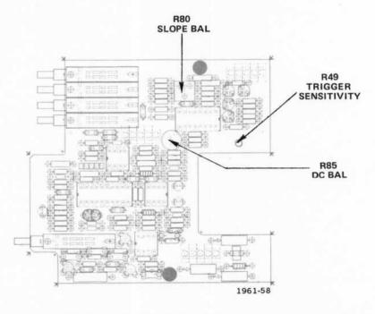
Fig. 8-12. Location of Triggering adjustments.
