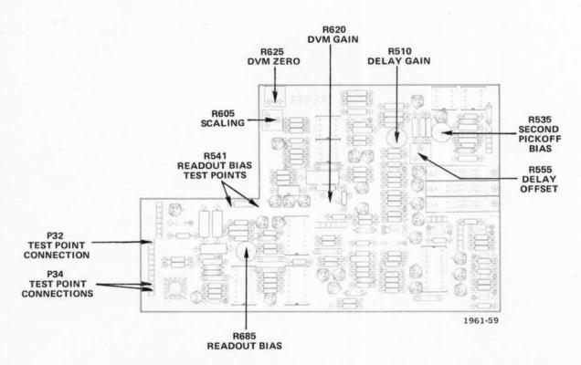
Fig. 8-13B. (SN B088749 & Below) Location of Digital Voltmeter adjustments.
