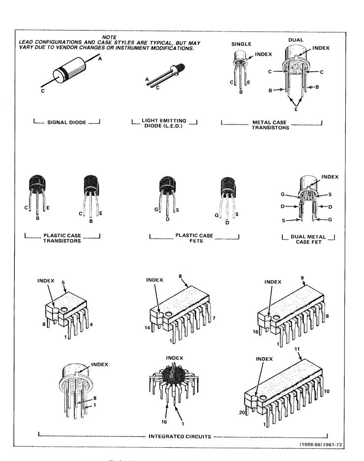
Fig. 8-1. Semiconductor lead configurations.
