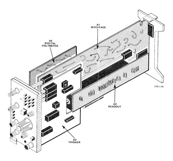
Fig. 8-2. Location of circuit boards in the 7B85.
