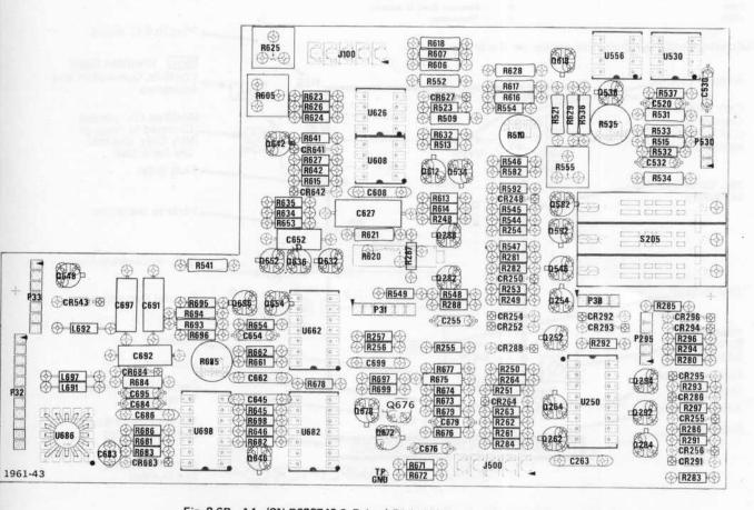
Fig. 8-6B. A4-(SN B088749 & Below) Digital Voltmeter circuit board assembly.
