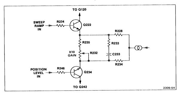
Fig. 5-4b. Simplified schematic of the X10 horizontal preamplifier.
