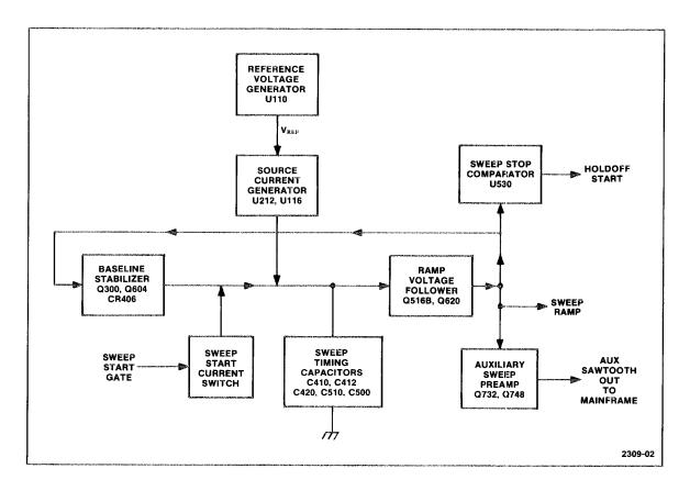
Fig. 5-2. Sweep generator block diagram.
