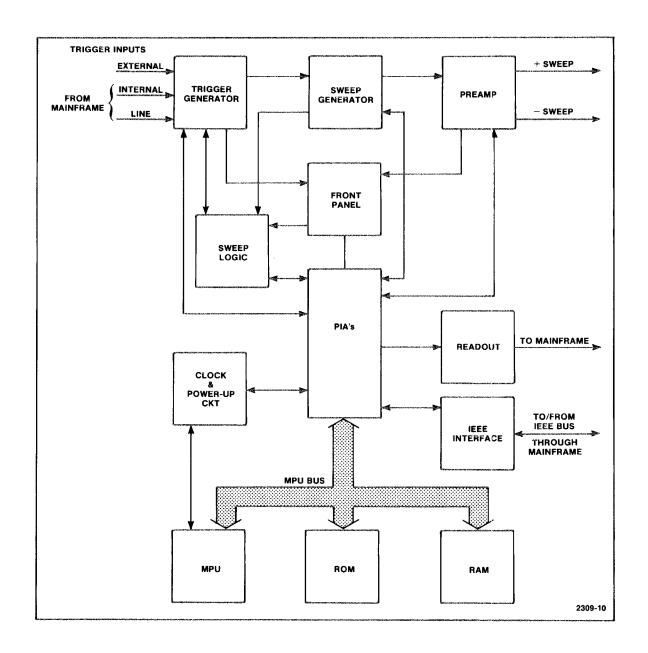
Fig. 1-1. Block diagram of the 7B90P.
