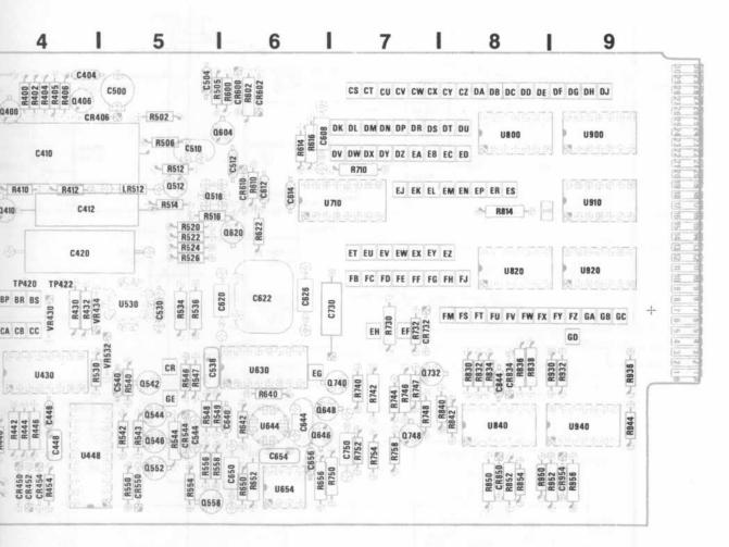
Fig. 8-4. P/O Sweep Board A20.
