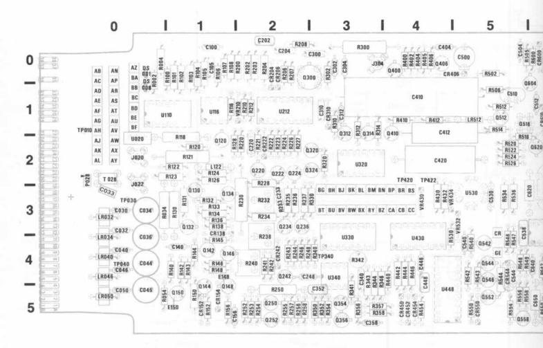
Fig. 8-4. P/O Sweep Board A20.
