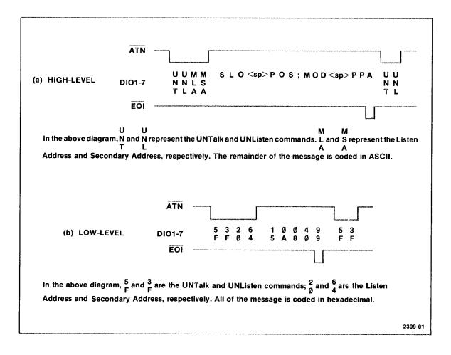
Fig. 3-4. Status of the ATN, ROI, and DIO signal lines during a high-level (a) and low-level (b) Set message.
