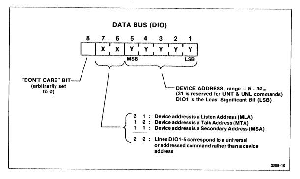
Fig. 3-3. Interpretation of the Data Bus (DIO1-8) when ATN is asserted.
