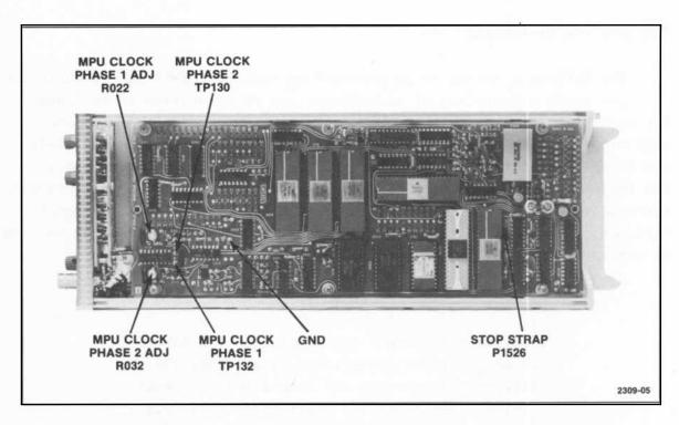
Fig. 6-1a. Test point and adjustment locations horizontal programming board.
