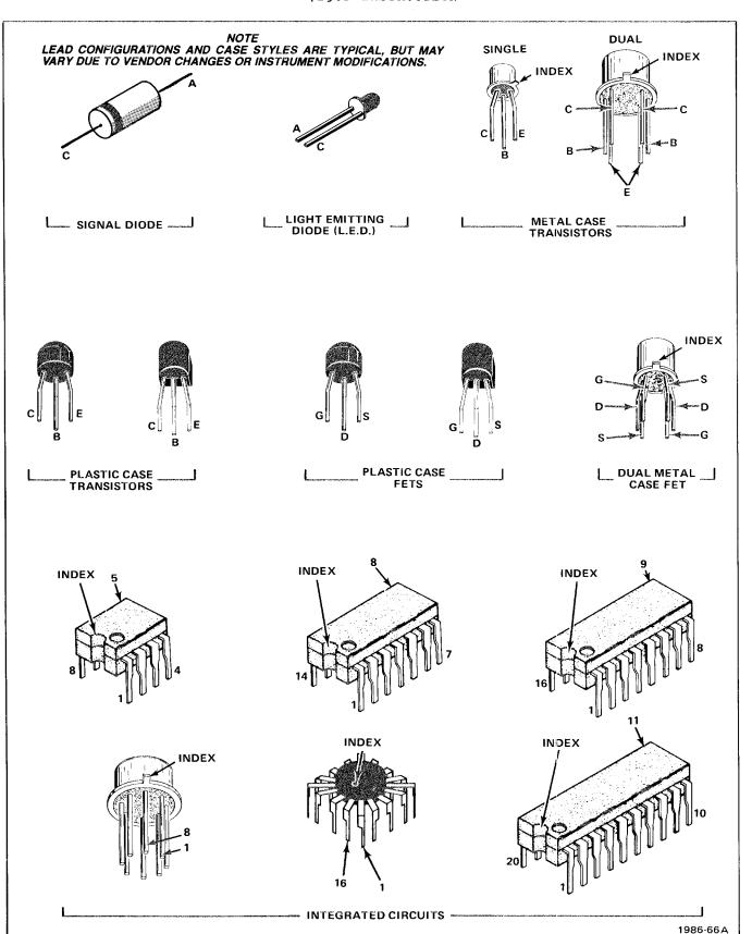
Fig. 4-15. Semiconductor lead configurations.
