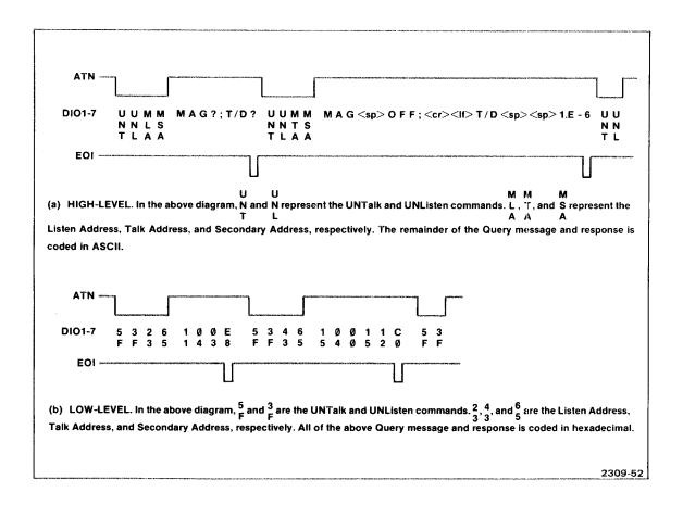
Fig. 3-5. Status of the ATN, EOI, and DIO signal lines during a highlevel (a) and low-level (b) Query message and response.
