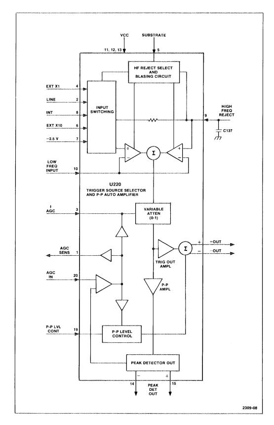
Fig. 5-6. Block diagram of U220.
