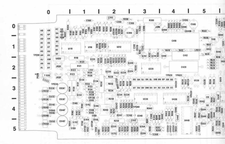
Fig. 8-2. P/O Sweep Board A20.
