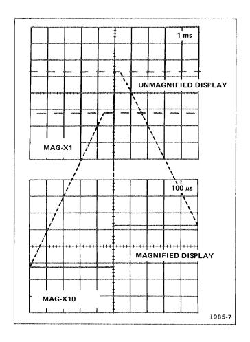
Fig. 2-3. Operation of the sweep magnifier.
