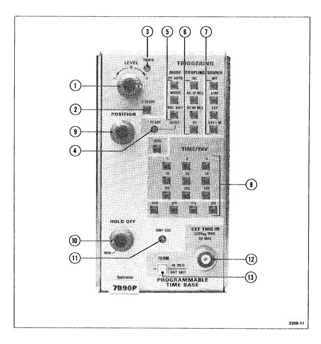
Fig. 2-1. Front panel of the 7B90P.
