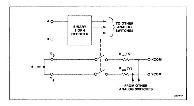
Fig. 5-3. Partial block diagram of the analog multiplexer, U212.
