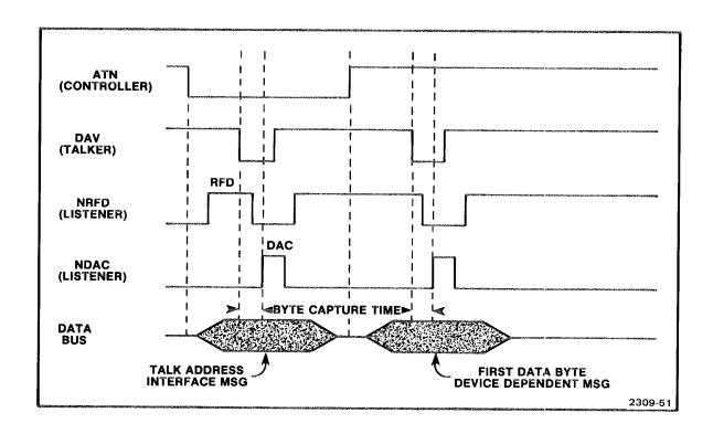
Fig. 3-2. A typical handshake sequence.
