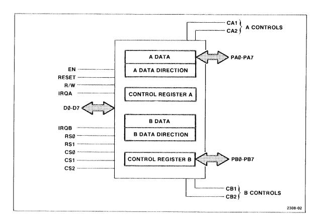
Fig. 5-8. Block diagram of the M6820 PIA.
