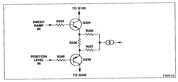
Fig. 5-4a. Simplified schematic of the X1 horizontal preamplifier.
