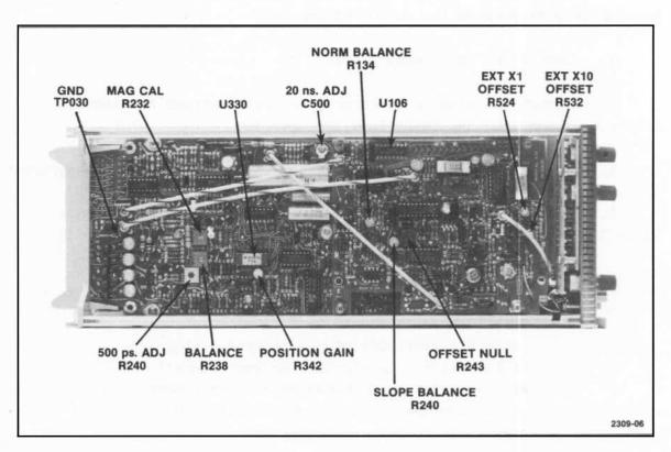
Fig. 6-1b. Test point and adjustment locations sweep and trigger boards.
