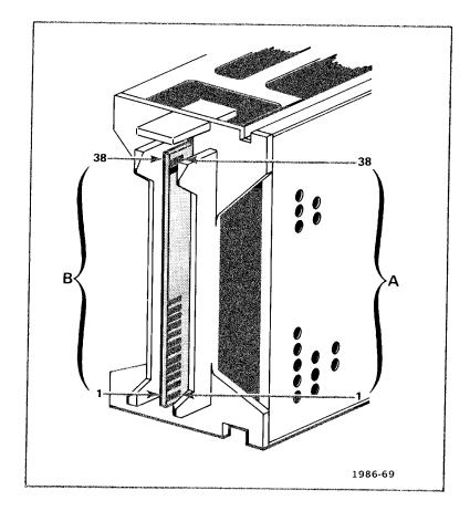
Fig. 4-2. Location of pin numbers on interface connector.
