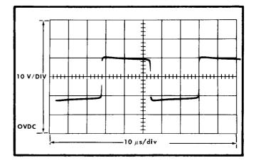
Fig. 4-3. Signal at Test Point 5, base of Q65 or Q75.
