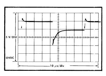
Fig. 4-2. Signal at Test Point 4, collector of Q65 or Q75.
