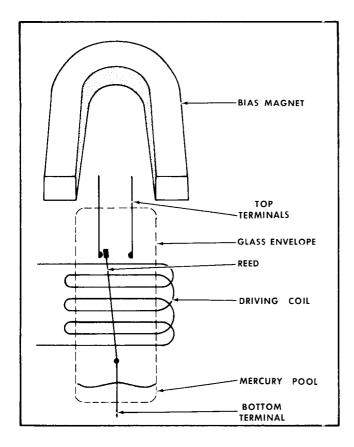
Fig. 3-2. Reed switch assembly, phantom view.
