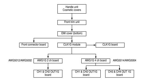
Figure 4-2: Disassembly procedures for internal modules (bottom)
