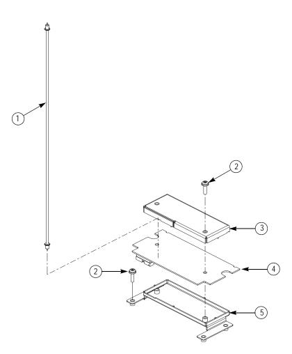
Figure 5-12: Exploded diagram - CLK1G module
