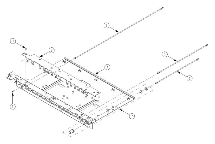
Figure 5-14: Exploded diagram - BNC bracket
