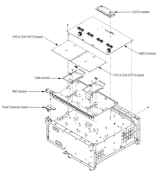
Figure 4-14: Front Connector board, CLK1G module, AWG1G board, and OUT1G boards removal (4-channel model)
