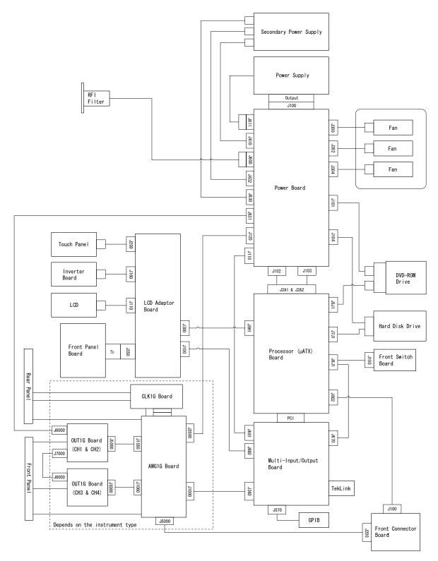
Figure 2-1: AWG5000 Series block diagram
