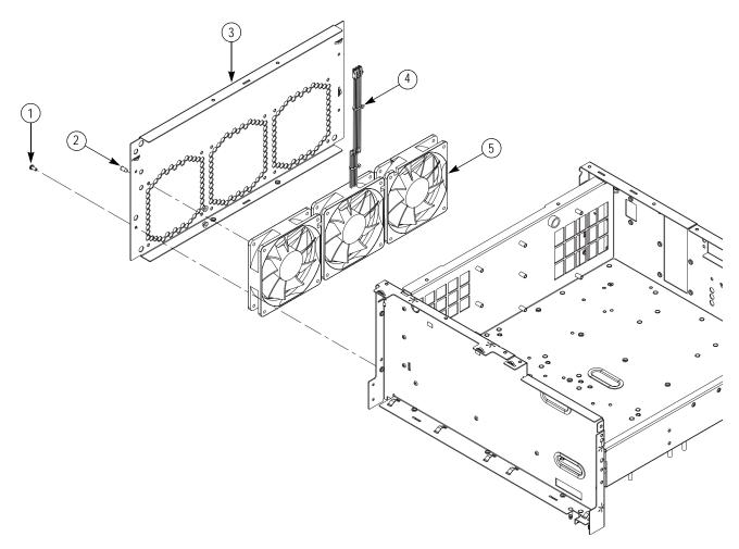
Figure 5-9: Exploded diagram - Fan tray assembly
