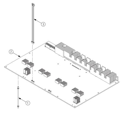
Figure 5-13: Exploded diagram - AWG1G module
