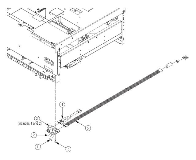
Figure 5-10: Exploded diagram - USB module
