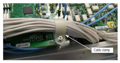
Figure 4-17: Location of the cable clamp on the AWG1G board
