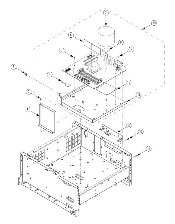
Figure 5-6: Exploded diagram - Processor module
