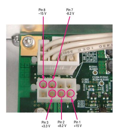
Figure 4-25: OUT1G board test points (J7000)
