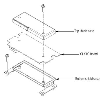
Figure 4-15: Disassembly of the CLK1G module
