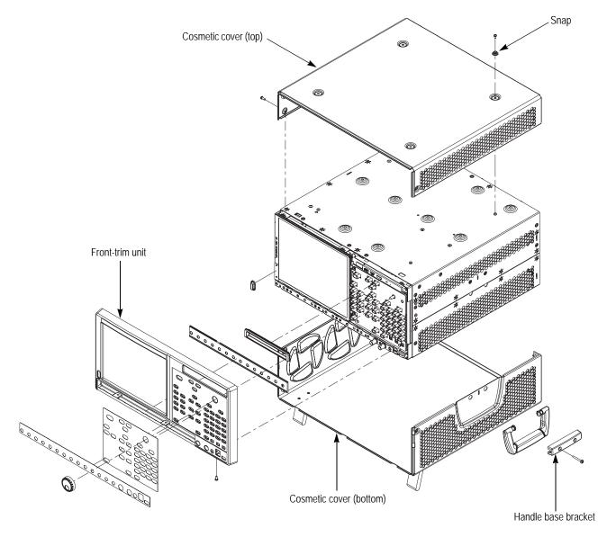
Figure 4-3: Handle, snaps, cosmetic covers, and front-trim unit removal
