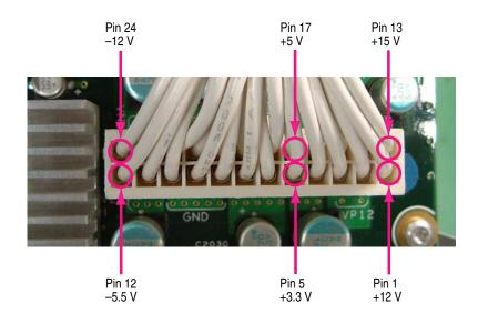
Figure 4-24: AWG1G board test points (J2000)
