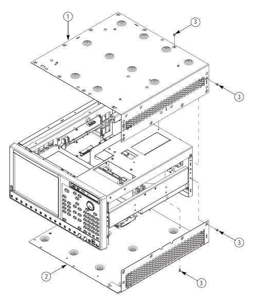
Figure 5-2: Exploded diagram - EMI Covers
