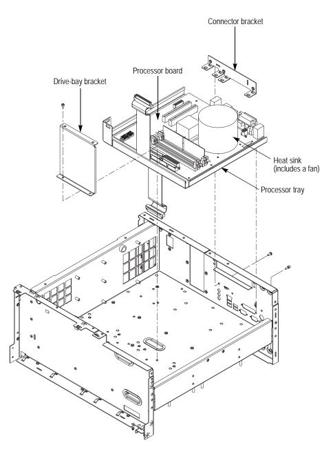
Figure 4-11: Processor board removal
