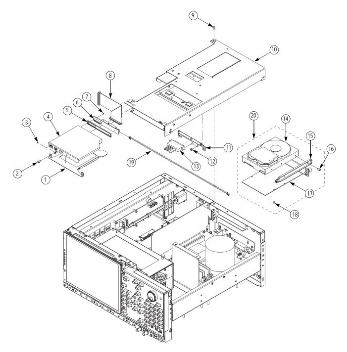
Figure 5-5: Exploded diagram - Drive module
