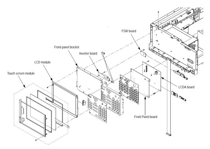
Figure 4-6: Disassembly of front-panel assembly
