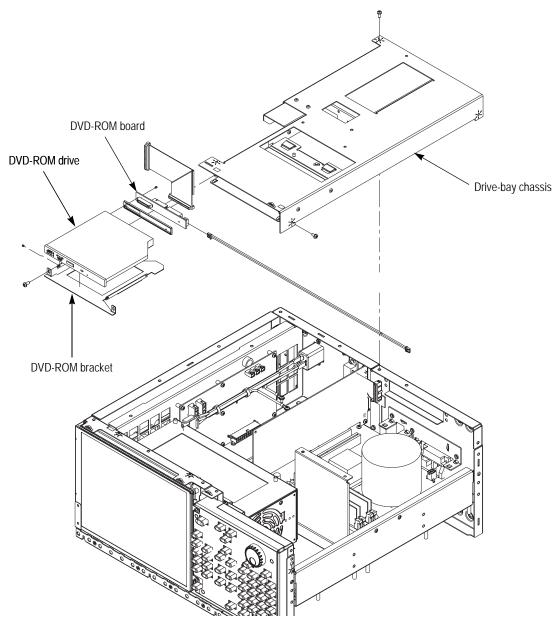
Figure 4-8: Drive module removal
