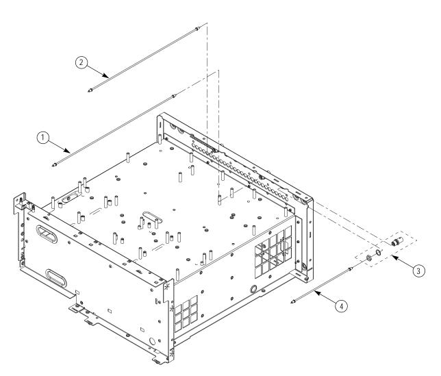
Figure 5-15: Exploded diagram - Rear connectors
