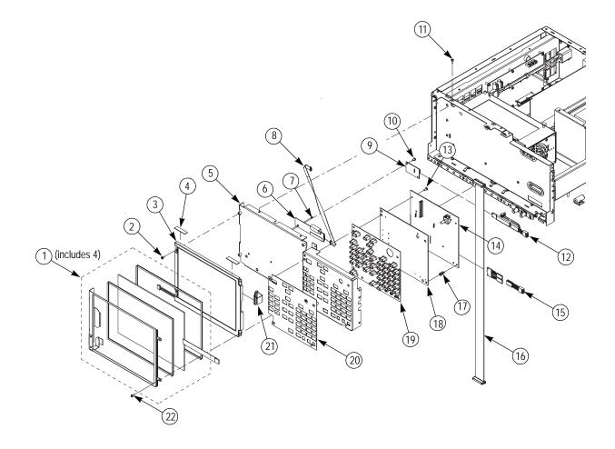
Figure 5-4: Exploded diagram - Front-panel assembly
