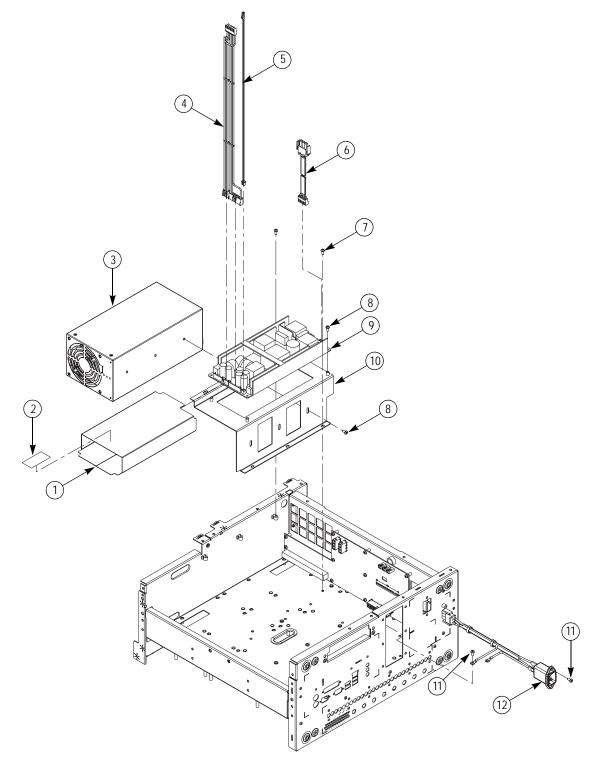
Figure 5-7: Exploded diagram - Power supply assembly
