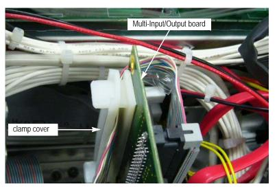
Figure 4-9: Removing the clamp cover
