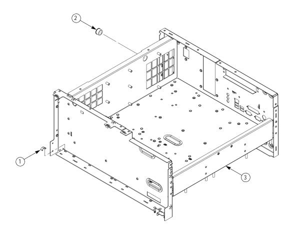
Figure 5-3: Exploded diagram - Chassis assembly
