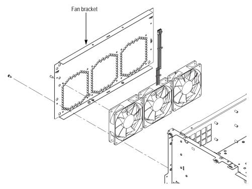
Figure 4-5: Fan tray unit removal
