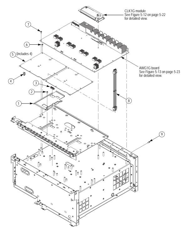
Figure 5-11: Exploded diagram - AWG1G/CLK1G/OUT1G modules
