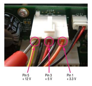
Figure 4-22: PWR board test points (J104)
