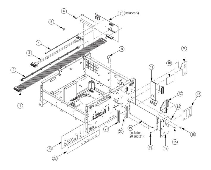
Figure 5-8: Exploded diagram - PCI/power interface module
