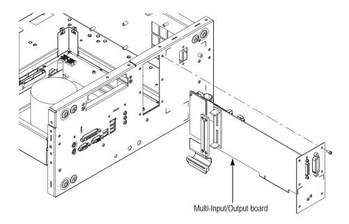
Figure 4-10: Multi-Input/Output board removal
