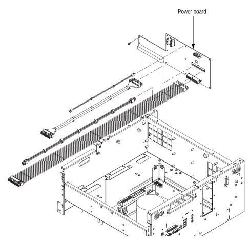
Figure 4-13: Power board removal
