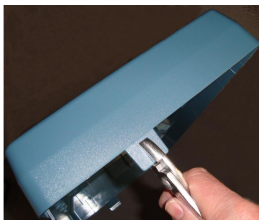
Figure 3: Removing tabs from the front protective cover
