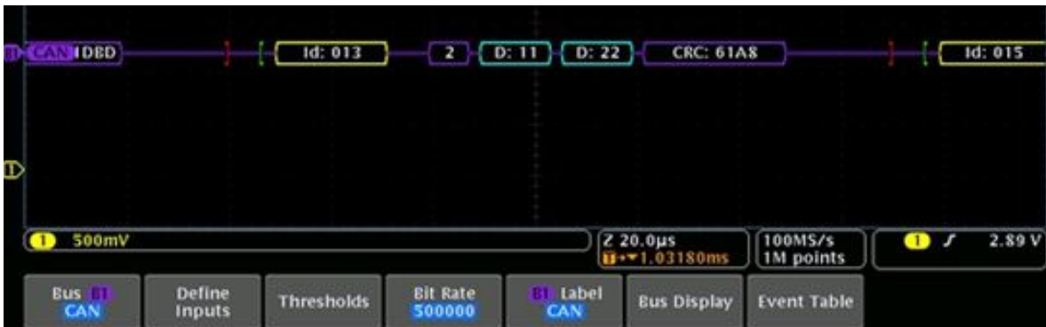
Color-coded display of a CAN bus, showing Start, DLC, Data, CRC, and Stop components of the serial signal.
