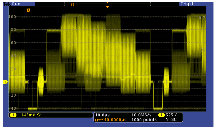
Viewing an NTSC video signal. Notice the intensity-graded view provided by the MDO's ability to represent time, amplitude, and distribution over time.
