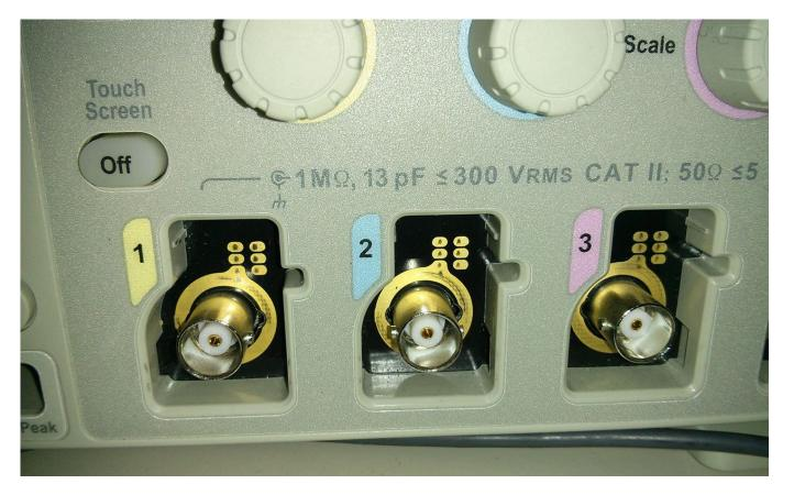
The scopes with the TekVPI interface are the MSO/DPO2000/3000/4000/5000/7000
