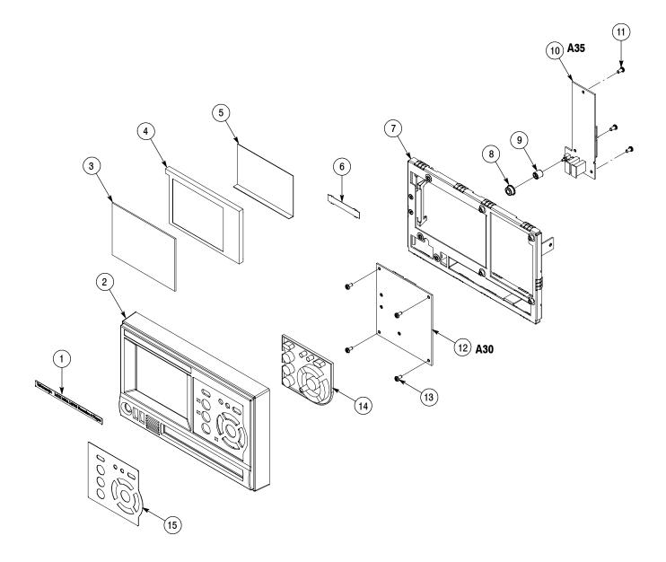
Figure 7-4: Front panel unit
