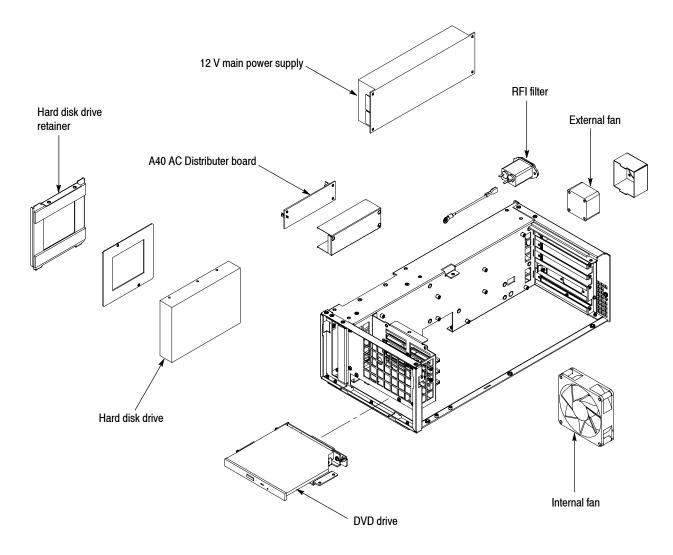
Figure 4-4: Internal modules
