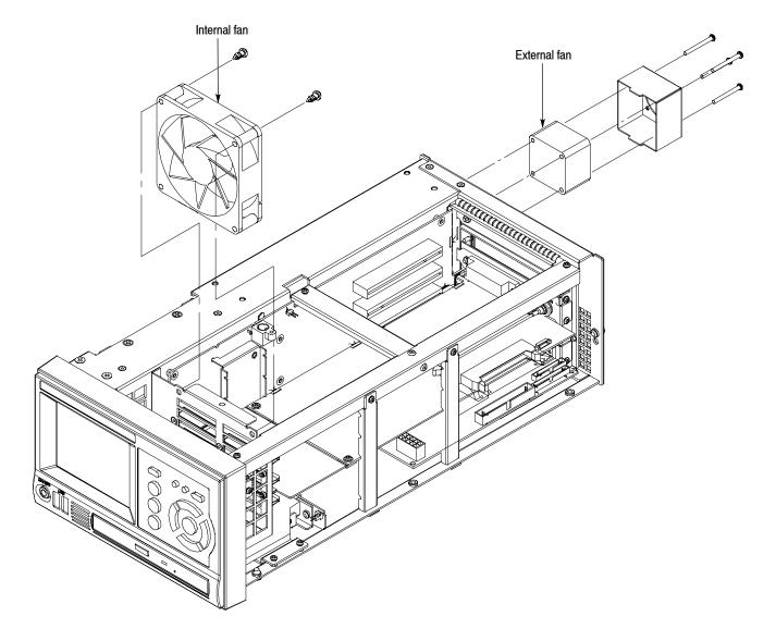
6. *Reinstallation:* Perform step 5 in reverse order to reinstall the external fan.
