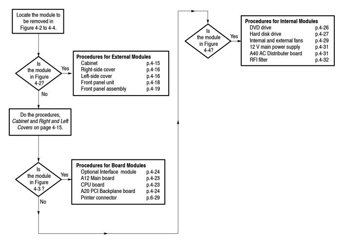
Figure 4-5: Guide to removal procedures
