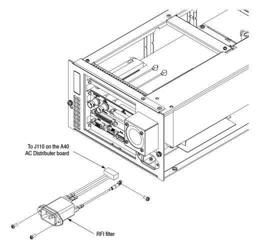
Figure 4-15: RFI filter removal
