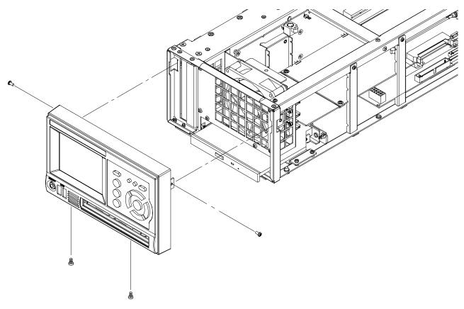
Figure 4-8: Front-panel unit removal
