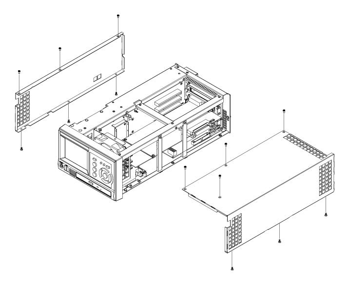
Figure 4-7: Right-side and left-side covers removal
