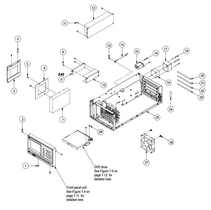
Figure 7-2: Internal modules (1)
