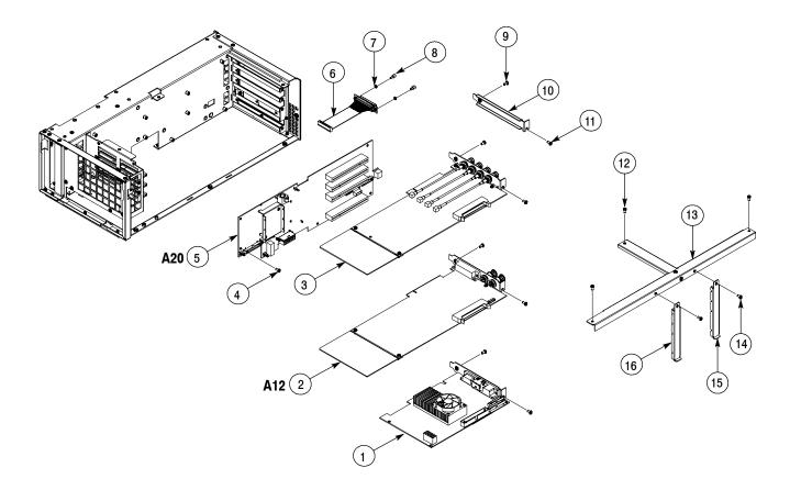
Figure 7-3: Internal modules (2)
