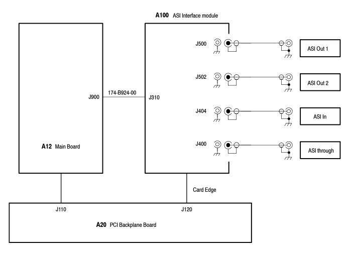
Figure 6-3: A100 ASI Interface module connections
