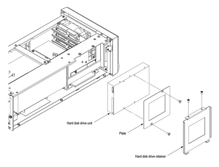
Figure 4-12: Hard disk drive removal
