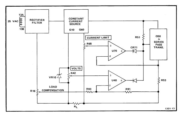
Fig. 3-1. Simplified diagram of PS 501 (-1, -2).
