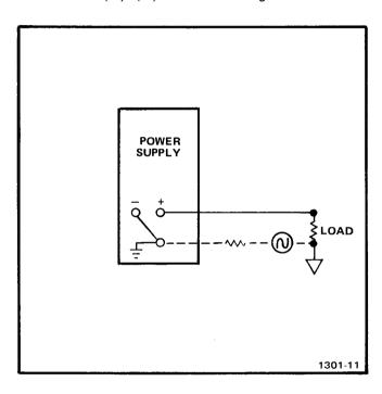
Fig. 2-10. Ground-loop current caused by remote grounded load.
