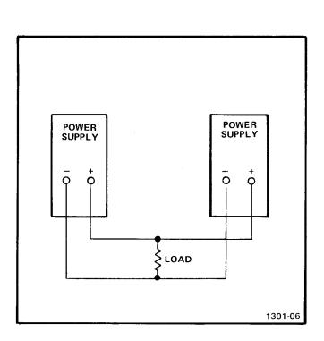
Fig. 2-5. Parallel-connected supplies.
