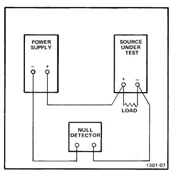
Fig. 2-6. Differential measurement connections.
