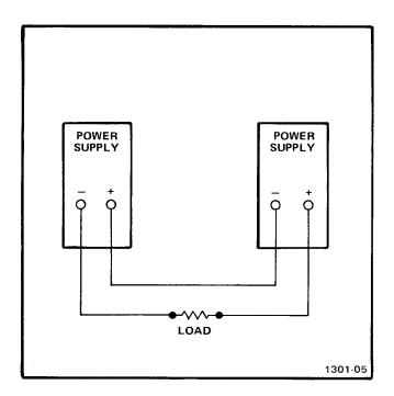
Fig. 2-4. Series-connected supplies.
