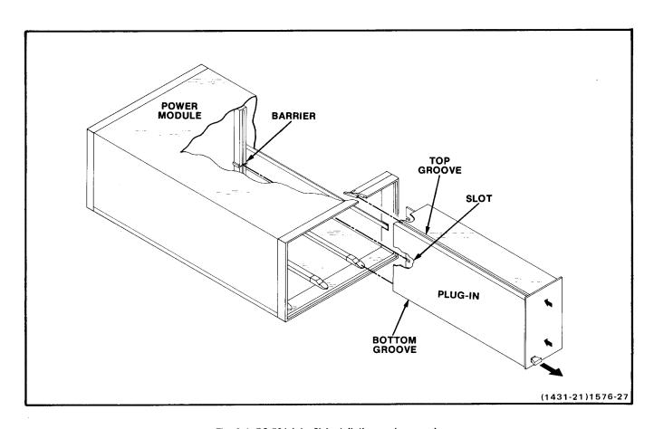
Fig. 2-1. PS 501 (-1, -2) Installation and removal.
