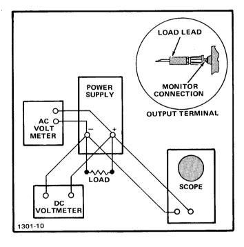
Fig. 2-9. Monitor connections.
