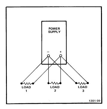
Fig. 2-8. Multiple load connections.
