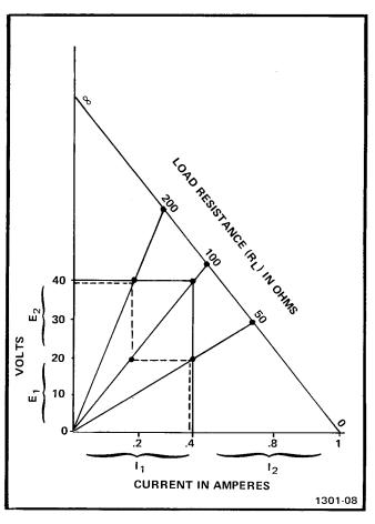
Fig. 2-7. Stair-step output characteristics of series and parallel connected supplies.
