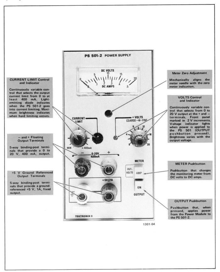
Fig. 2-3. Controls and Connectors.
