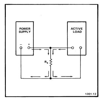
Fig. 2-11. Reverse-current shunt (R<sub>s</sub>) with active load.
