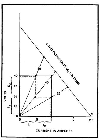
Fig. 1-7. Output characteristics with various currents, voltages, and loads.
