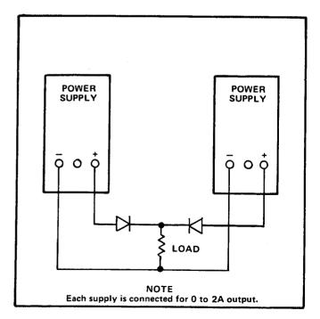
Fig. 1-9. Supplies parallel-connected.
