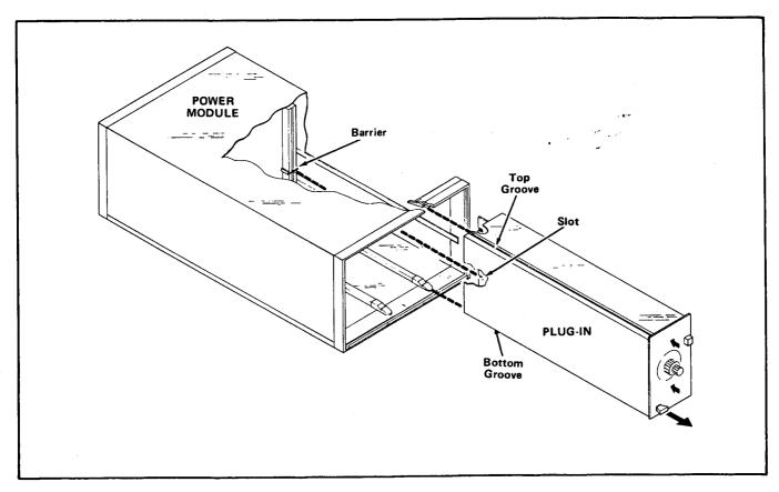
Fig. 1-2. Plug-in module installation/removal.
