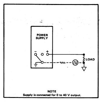
Fig. 1-5. Ground loop created by grounded remote lead.
