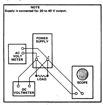
Fig. 1-4. Monitor and load connections.
