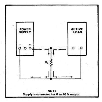
Fig. 1-6. Reverse current shunt (Rs) with active load.
