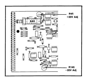
Fig. 3-1. Location of +20 V and -20 V adjustment.
