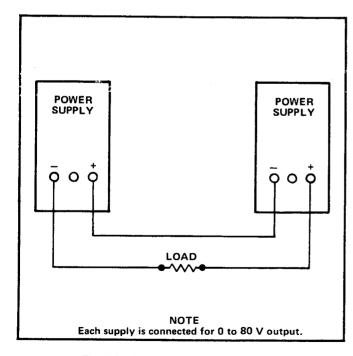
Fig. 1-8. Supplies series-connected.
