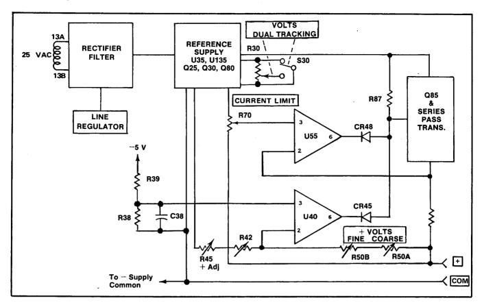
Fig. 5-1. Simplified block diagram of PS 503A.
