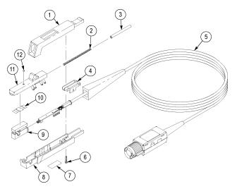
Figure 27: TCP202 and Replaceable Parts and Accessories
