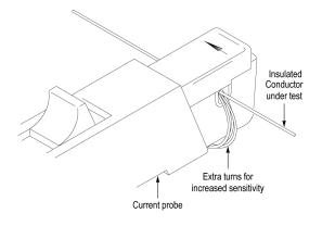
Figure 7: Increasing Probe Sensitivity
