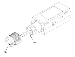
Figure 19: Replacing the TekProbe collar
