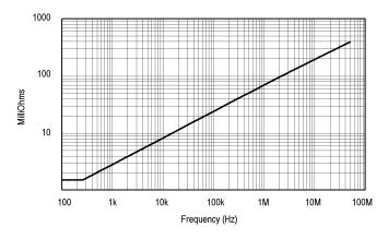
Figure 13: Insertion Impedance - Magnitude - Single Conductor
