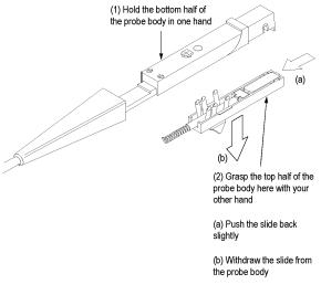
Figure 25: Removing the Probe Slide
