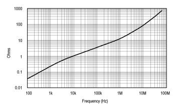
Figure 15: Insertion Impedance - Magnitude - 10-Turn #24 AWG Primary
