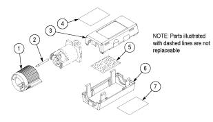
Figure 28: Replaceable Parts - Compensation Box
