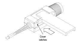
Figure 20: Removing the Compensation Box Covers
