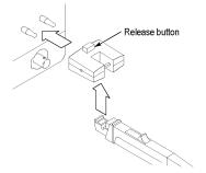
Figure 3: Connecting the Calibrator
