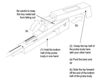
Figure 24: Removing the Top Half of the Probe
