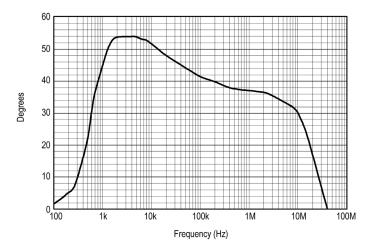
Figure 14: Insertion Impedance - Phase Angle - Single Conductor
