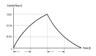
Figure 11: High-Impedance Source Current Ramp
