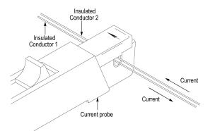
Figure 5: Measuring Differential Current and Nulls
