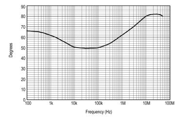
Figure 16: Insertion Impedance - Phase Angle - 10-Turn #24 AWG Primary
