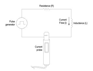
Figure 10: Measuring Inductance with a High-Impedance Source
