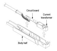
Figure 26: Removing the Current Transformer
