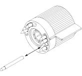
Figure 18: Replacing TekProbe Interface Pins
