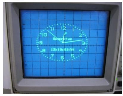
You can turn your old analog scope into a clock using a simple microcontroller circuit.
