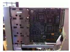
To my disappointment, unlike other Tektronix oscilloscope models, this acquisition board is also the mainboard of the oscilloscope and is very compact with mostly surface-mounted components. There are
