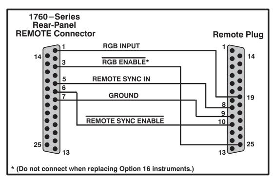
**Figure B-2.** Using the 1760–Series as a 1740/1750–Series replacement.
