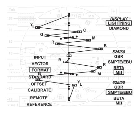
Figure 2-19. Lightning Display in MII Format.
