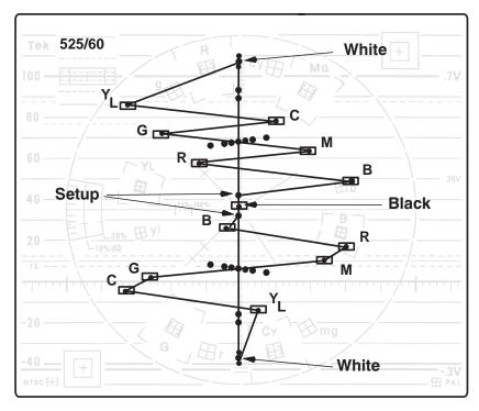
Figure 4-14. Lightning display showing correct timing.
