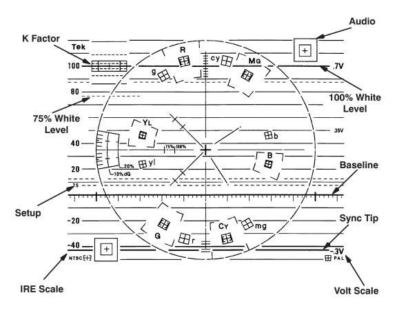
**Figure 4-3.** Dual Standard waveform/vector graticule.
