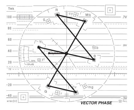
Figure 2-14. Vectorscope color bar display.
