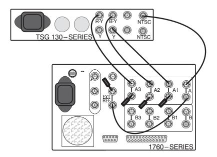
**Figure 2-4.** Equipment hook-up for Operator's Checkout Procedure.
