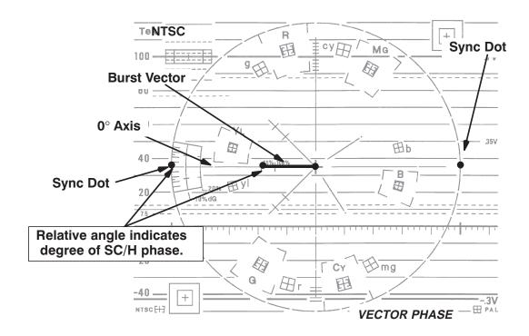
Figure 4-6. NTSC dual-dot SC/H display.
