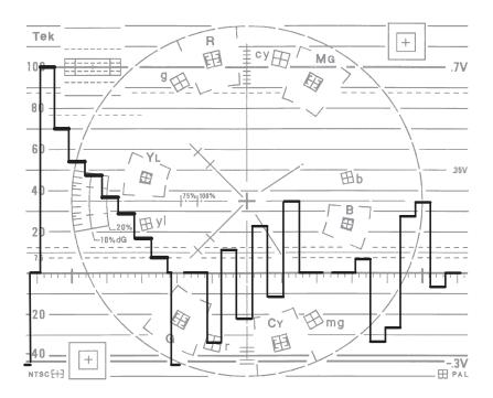
Figure 2-5. Component waveform display (A123).
