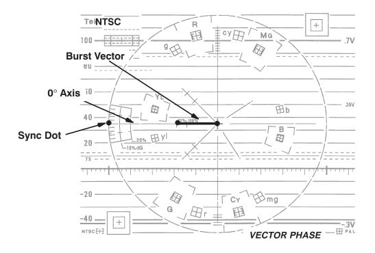
Figure 4-7. NTSC single-dot SC/H display.
