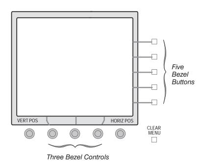
Figure 2-1. Multi-Use Bezel Controls and Buttons.
