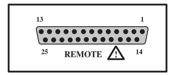
**Figure B-1.** Rear panel REMOTE connector.
