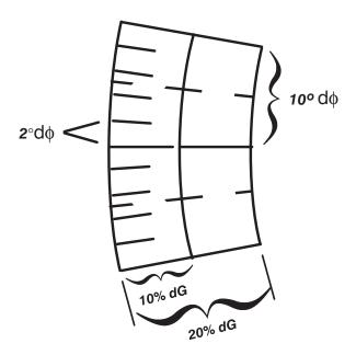
**Figure 4-5.** Differential gain and phase measurements.
