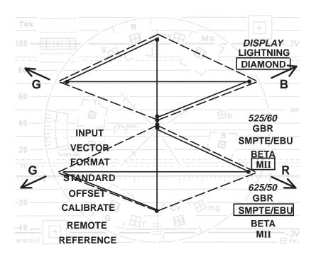
Figure 2-20. Diamond display, showing signal within gamut limit.
