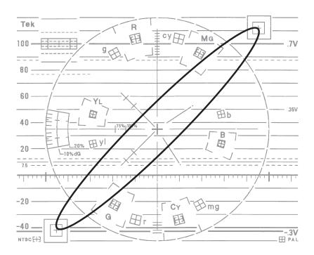
Figure 2-16. Audio display with phase error.
