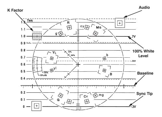
**Figure 4-2.** PAL waveform/vector graticule.
