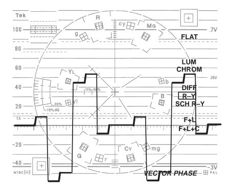
**Figure 2-10.** Two-Line R-Y display of color bar signal.
