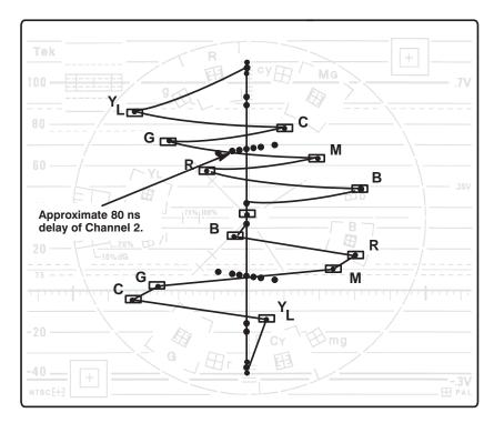
Figure 4-15. Lightning display showing delay.
