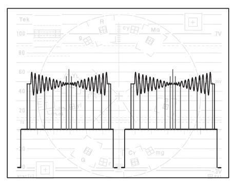
Figure 4-17. Bowtie display showing a sharp null.
