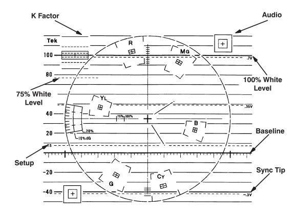
Figure 4-1. NTSC waveform/vector graticule.
