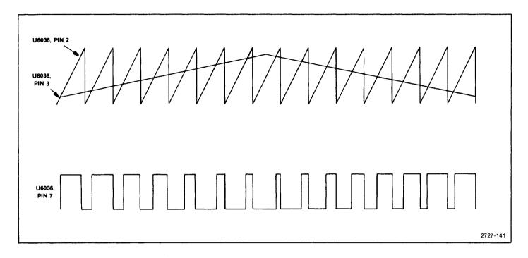
Figure 7-34. Primary regulator input and output waveforms.
