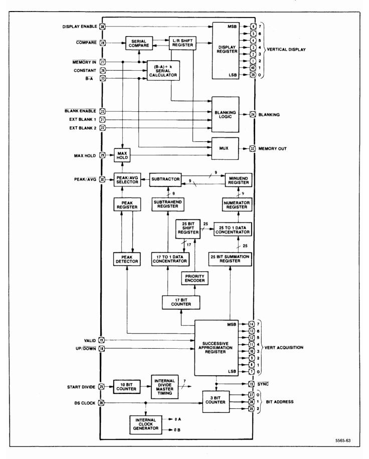
Figure 7-15. Vertical control IC block diagram.
