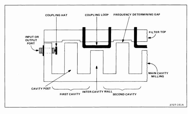
Figure 7-1. Cross section of a four-cavity filter.
