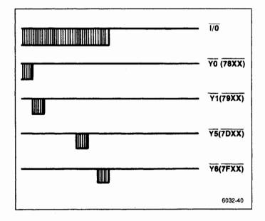
Figure 6-31. Chip selects Y0, Y1, Y5, and Y7 in relation to T/O.
