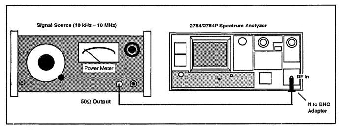
Figure A. Test equipment setup for measuring 10 kHz to 10 MHz frequency response
