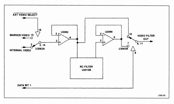
Figure 7-14. Simplified diagram of a video filter.
