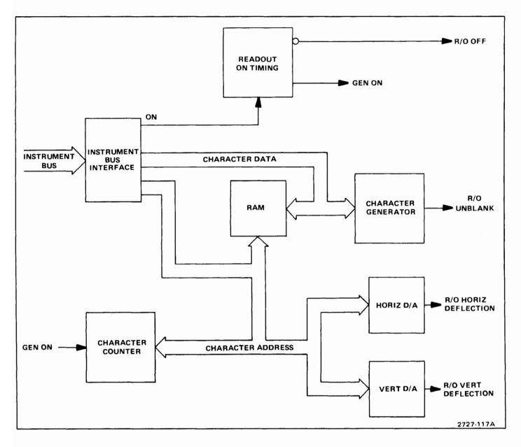
Figure 7-17. Block diagram of crt readout.
