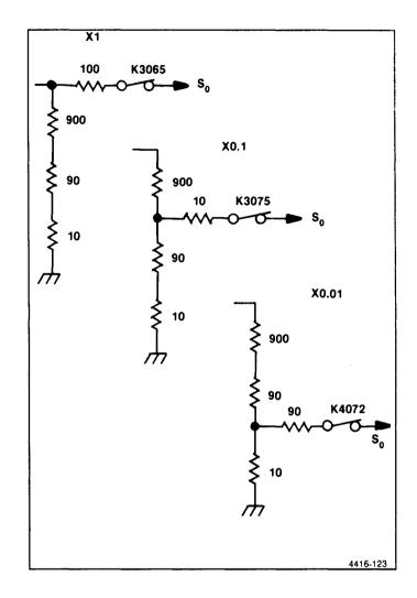
Figure 7-24. Simplified span decade attenuator.
