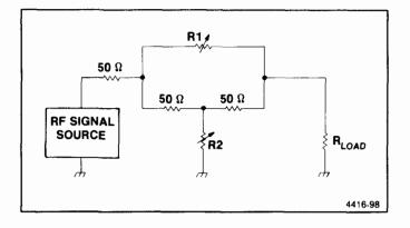
Figure 7-7. Bridged "T" attenuator equivalent circuit.
