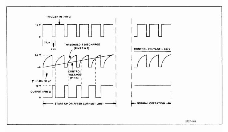
Figure 7-35. Timing waveforms for soft-start circuit.
