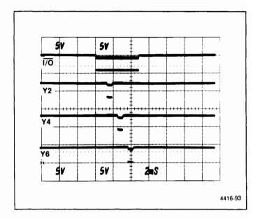
Figure 6-32. Chip selects Y2, Y4, and Y6 in relation to 1/O.
