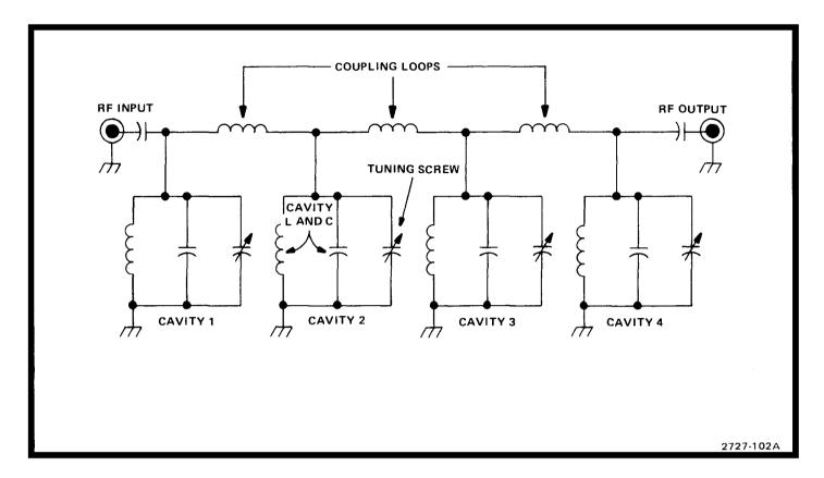
Figure 7-2. Equivalent circuit of the four-cavity filter.
