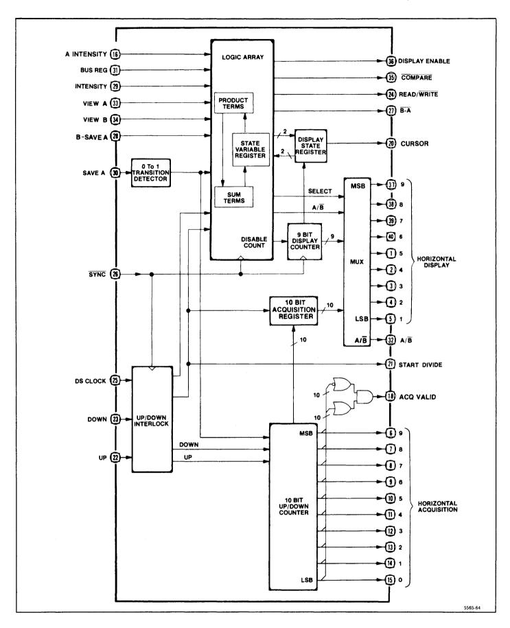
Figure 7-16. Horizontal control IC block diagram.
