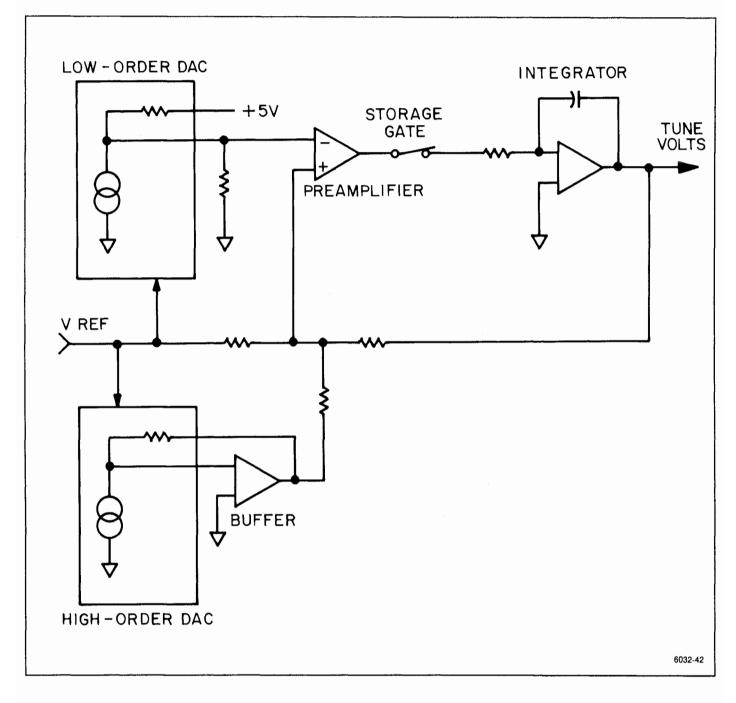
Figure 7-26. Simplified tune voltage converter.
