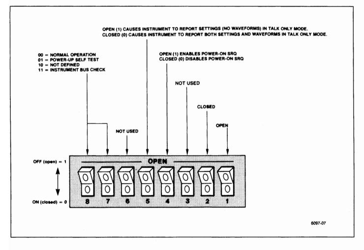
Figure 7-33. Options switch bank on the Memory board.
