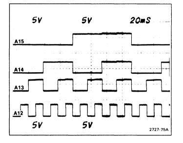
Figure 6-27. A15 through A12 in microcomputer test mode.
