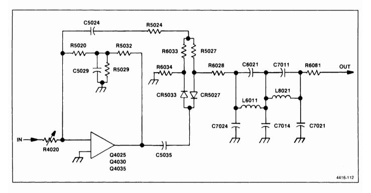
Figure 7-11. Simplified detector circuit.
