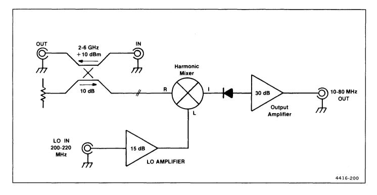
Figure 7-27. Simplified schematic of harmonic mixer.
