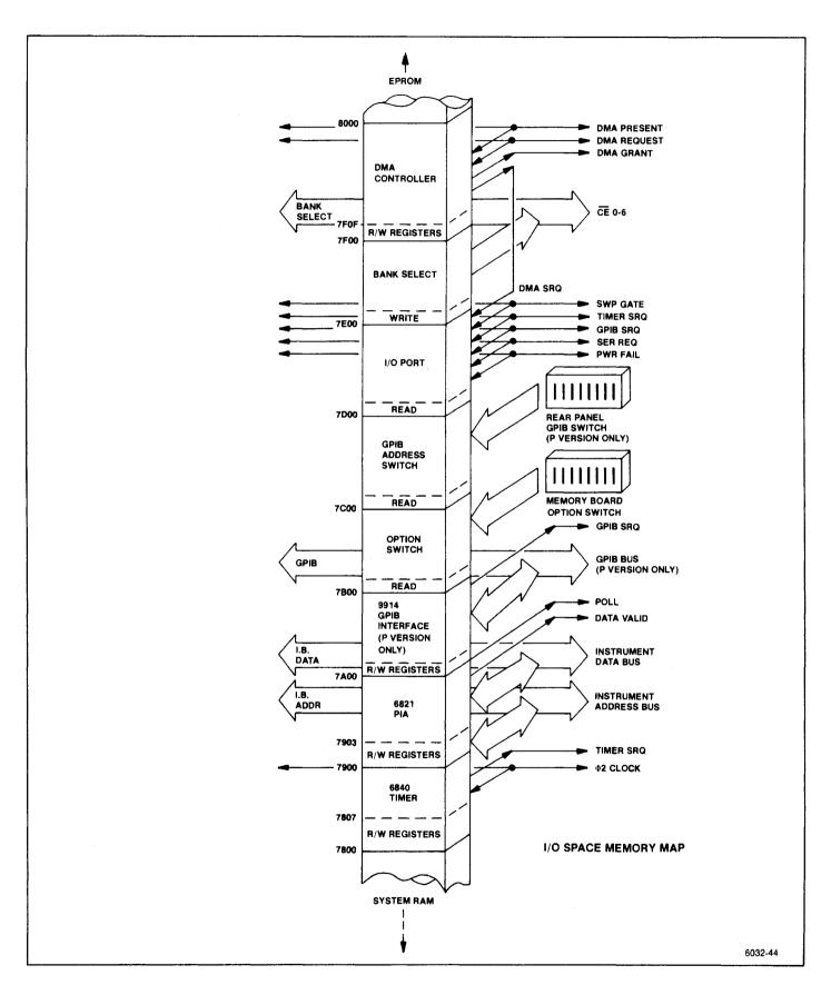
Figure 7-31. I/O address space.
