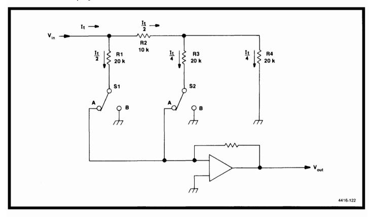
Figure 7-23. Simplified digital-to-analog converter.
