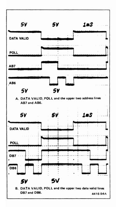
Figure 6-33. Instrument bus check.
