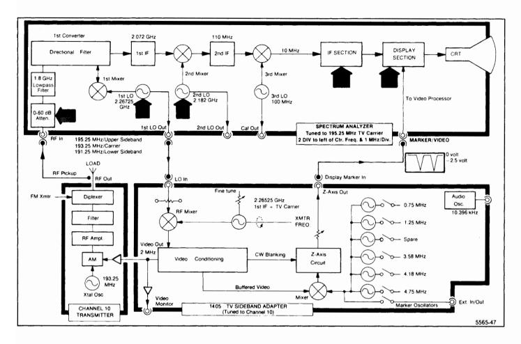
Figure 7-13. Functional diagram showing the Spectrum Analyzer and 1405 TV Sideband Adapter System.
