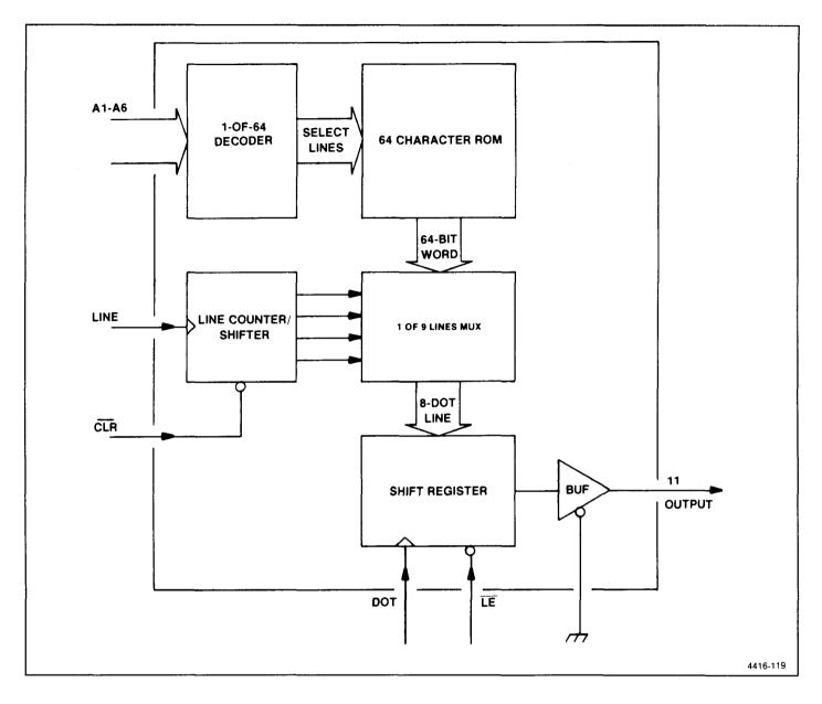
Figure 7-20. Character generator block diagram.
