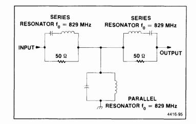
Figure 7-3. Simplified diplexer diagram.
