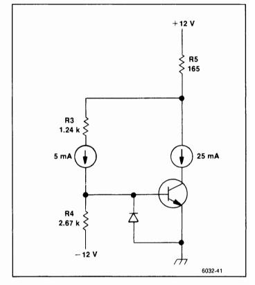
Figure 7-5. Equivalent dc circuit of an 829 MHz amplifier. 829 MHz 2nd Converter board (A23A7).
