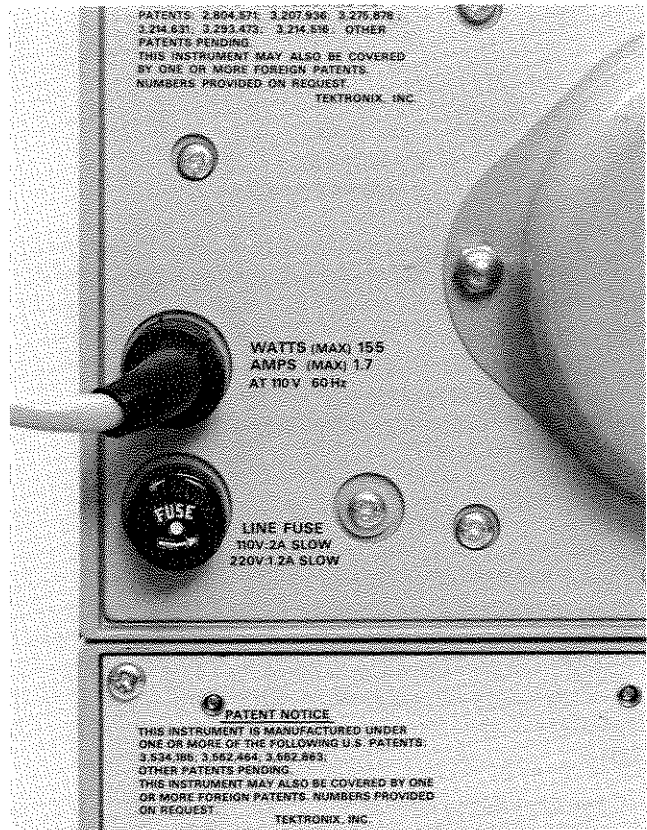
Fig. 1. Fuse location and fuse size information. See Electrical Parts List for part numbers and ordering information.
