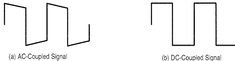
Figure 3–2: Effect of AC or DC Coupling on Low-Frequency Signals
