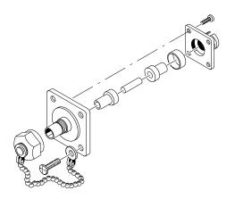
Figure H 4: DIN 47256 Optical Bulkhead Assembly
