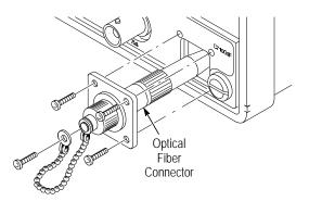
Figure H 1: Removing the Optical Bulkhead Connector
