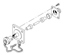
Figure H 3: ST Optical Bulkhead Assembly
