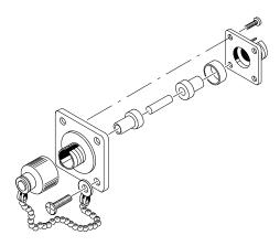
Figure H 2: FC Optical Bulkhead Assembly
