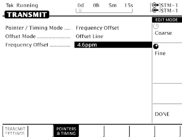
Figure 2 30: Adjusting Frequency Offset Using the Knob
