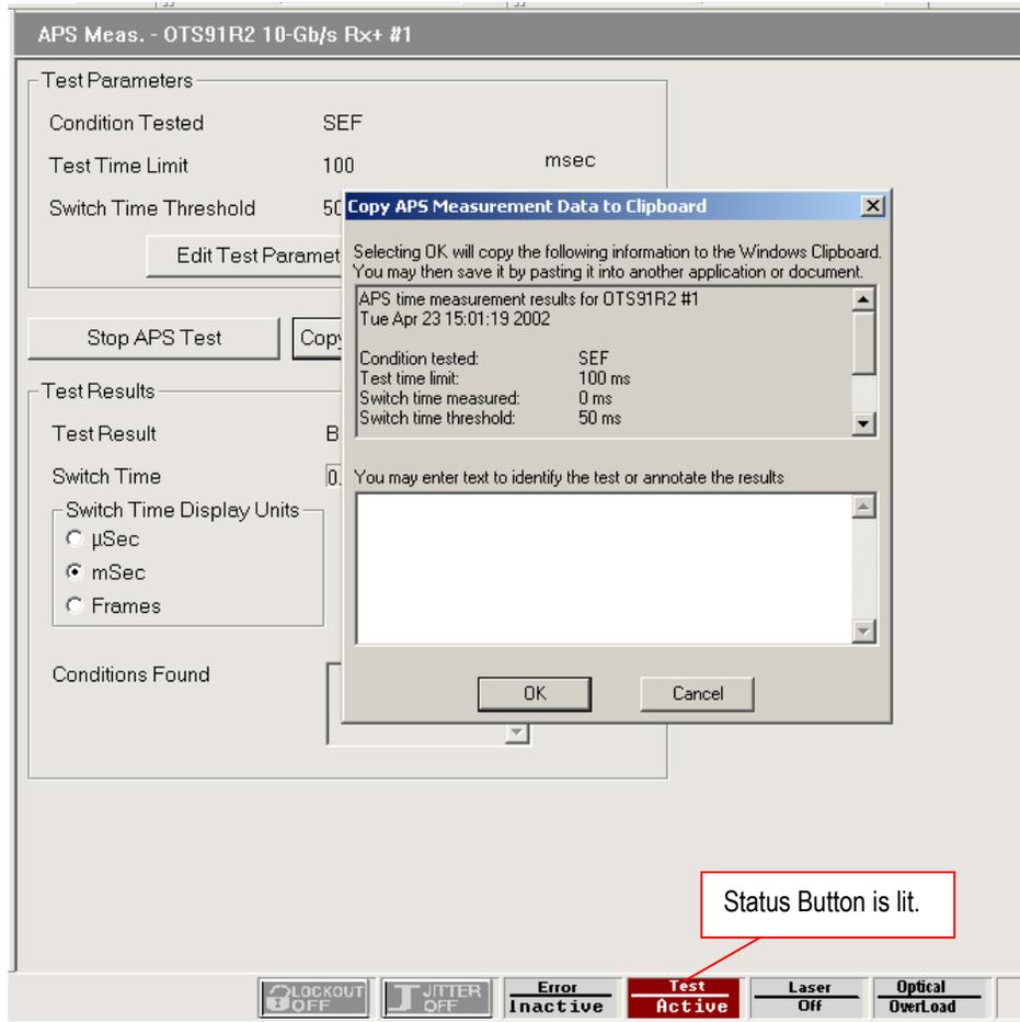
Figure 2-54: Copy APS Measurement Data dialog box
