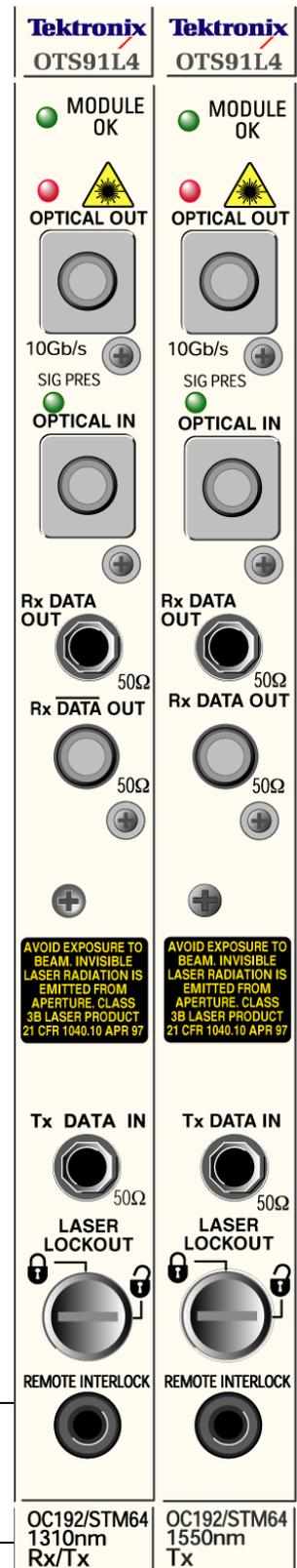
Figure B-1: Transceiver Front Panels
