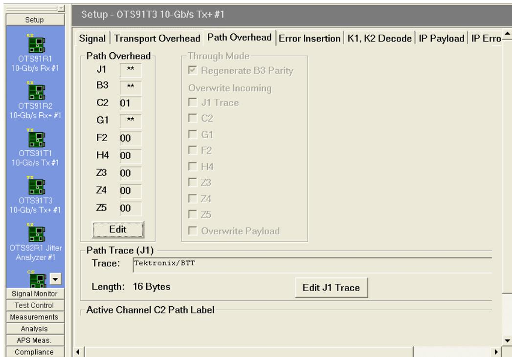
Figure 2-16: Transmitter – Path Overhead Property Menu
