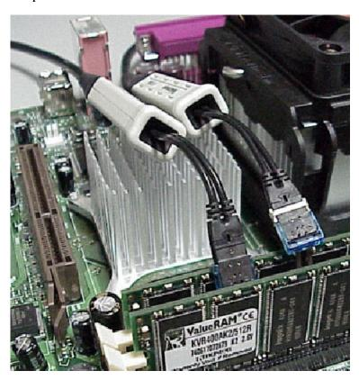
Figure 10: Soldered Tip-Clip assemblies
