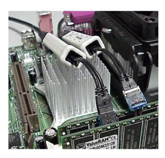
Figure 20: Circuit board with Tip-Clip assemblies
