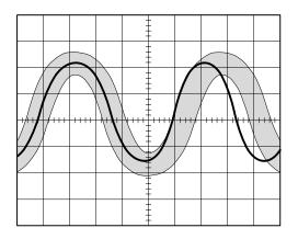
Figure 3–82: Comparing a Waveform to a Limit Template
