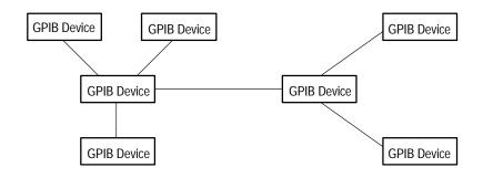
Figure 3–75: Typical GPIB Network Configuration
