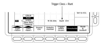
Figure 3–43: Pulse Trigger Readouts
