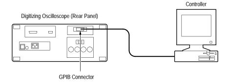
Figure 3–77: Connecting the Oscilloscope to a Controller
