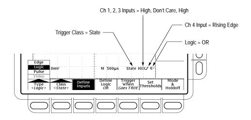
Figure 3–39: Logic Trigger Readouts — State Class Selected
