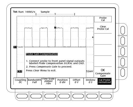
Figure 3–63: Probe Cal Menu and Gain Compensation Display
