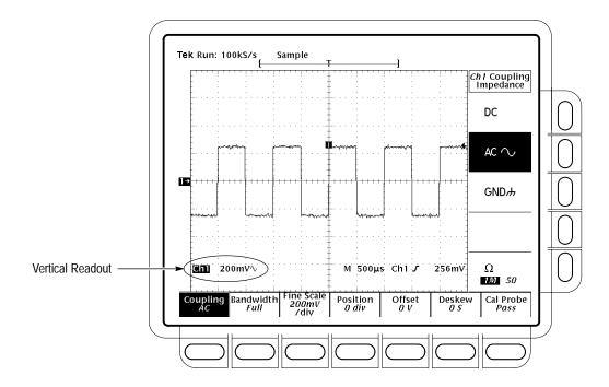
Figure 3-6: Vertical Readouts and Channel Menu
