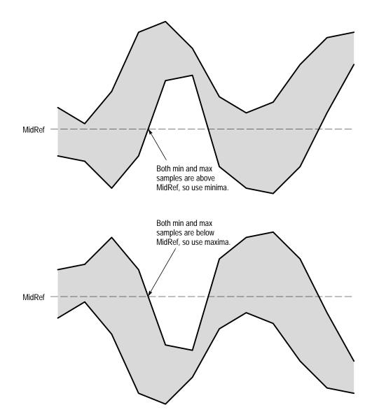
Figure B-4: Choosing Minima or Maxima to Use for Envelope Measurements
