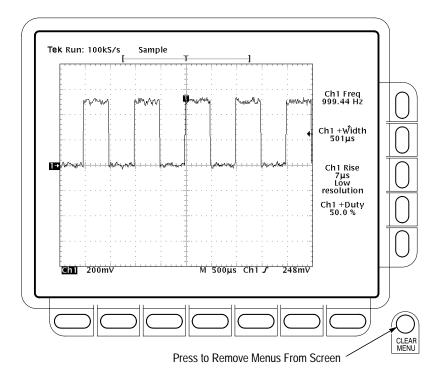
Figure 2–15: Four Simultaneous Measurement Readouts
