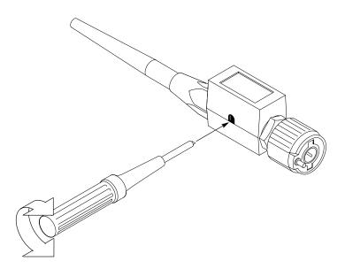
Figure 3–2: P6139A Probe Adjustment
