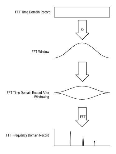
Figure 3–93: Windowing the FFT Time Domain Record
