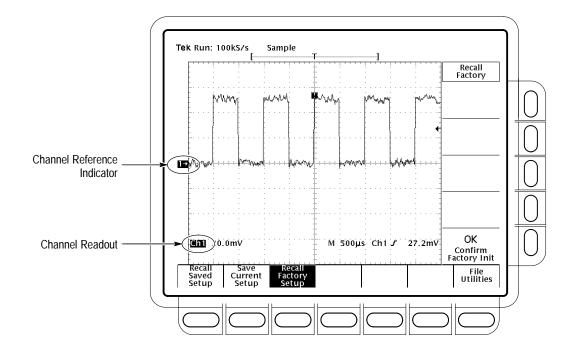
Figure 3–3: The Channel Readout
