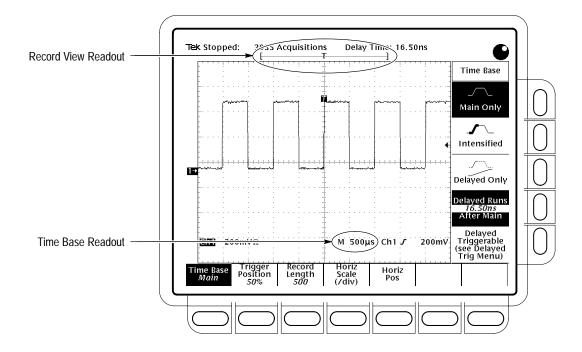
Figure 3–7: Record View and Time Base Readouts
