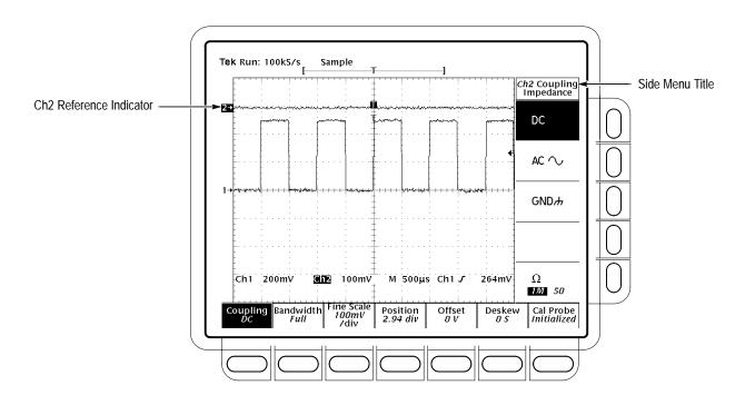
Figure 2–12: The Vertical Main Menu and Coupling Side Menu
