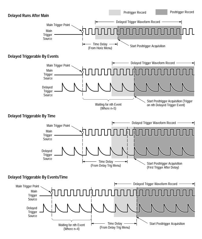
Figure 3–49: How the Delayed Triggers Work
