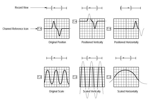
The Record View, at the top of the display, indicates where the trigger occurs and what part of the waveform record is displayed.
