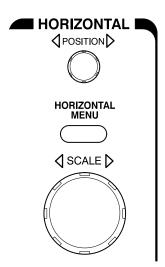
Figure 3–8: Horizontal Controls
