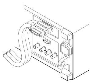
Figure 3–76: Stacking GPIB Connectors
