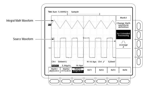
Figure 3–97: Integral Math Waveform
