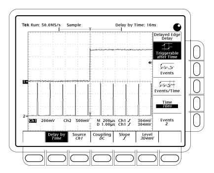
Figure 3–50: Delayed Trigger Menu
