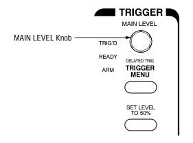
Figure 2–7: TRIGGER Controls
