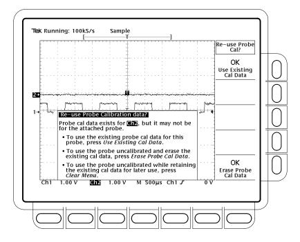
Figure 3-64: Re-use Probe Calibration Data Menu
