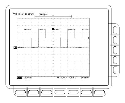
Figure 2–9 shows the display after pressing AUTOSET. If necessary, you can adjust the waveform now by using the knobs discussed earlier in this example.
