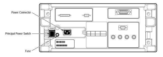
Figure 1–1: Rear Panel Controls Used in Start Up
