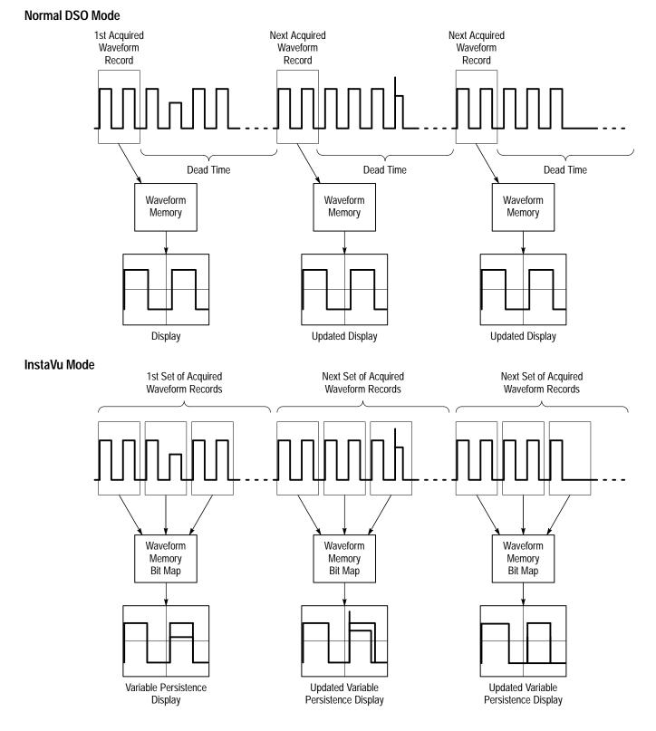
Figure 3–26: Normal DSO Acquisition and Display Mode Versus InstaVu Mode
