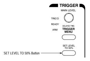
Figure 2–4: Trigger Controls
