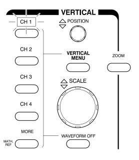
Figure 2–11: The Channel Buttons and Lights
