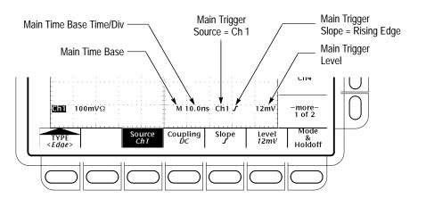
Figure 3–34: Example Trigger Readouts — Edge Trigger Selected
