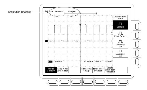
Figure 3–14: Acquisition Menu and Readout
