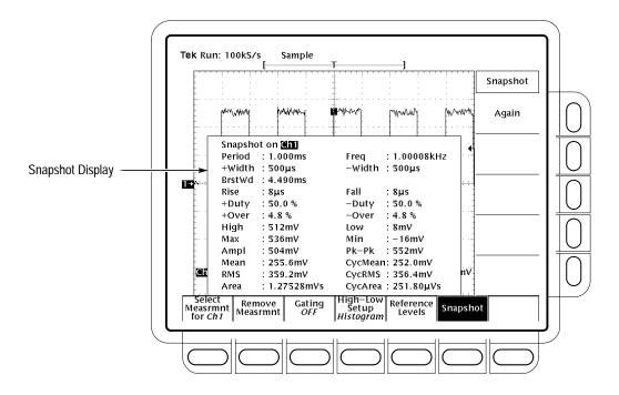
Figure 3–57: Snapshot Menu and Readout
