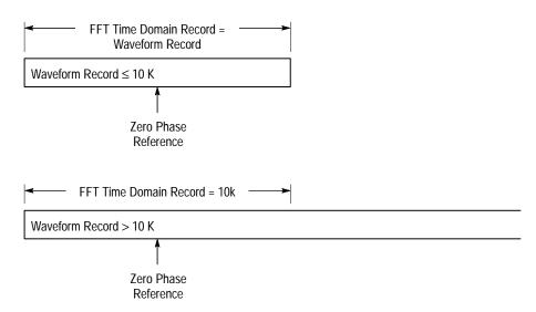
Figure 3–90: Waveform Record vs. FFT Time Domain Record
