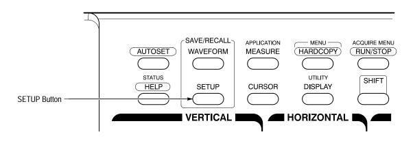
Figure 2–2: SETUP Button Location
