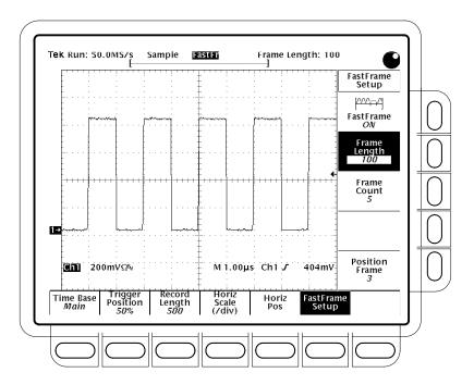
Figure 3–29: Horizontal Menu — FastFrame Setup
