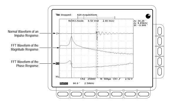
Figure 3–86: System Response to an Impulse
