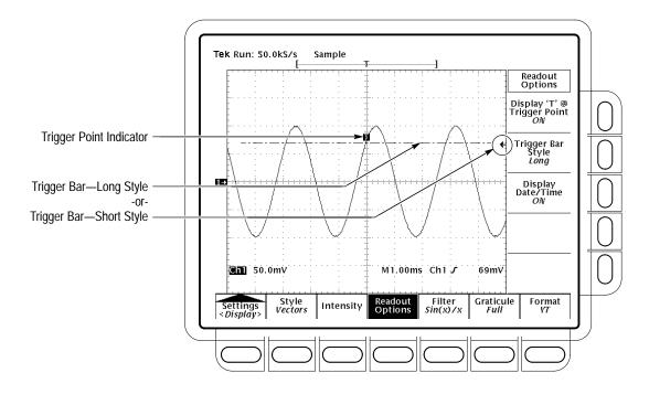
Figure 3–18: Trigger Point and Level Indicators
