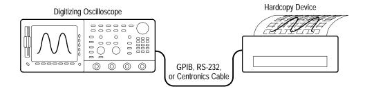
Figure 3–73: Connecting the Oscilloscope Directly to the Hardcopy Device
