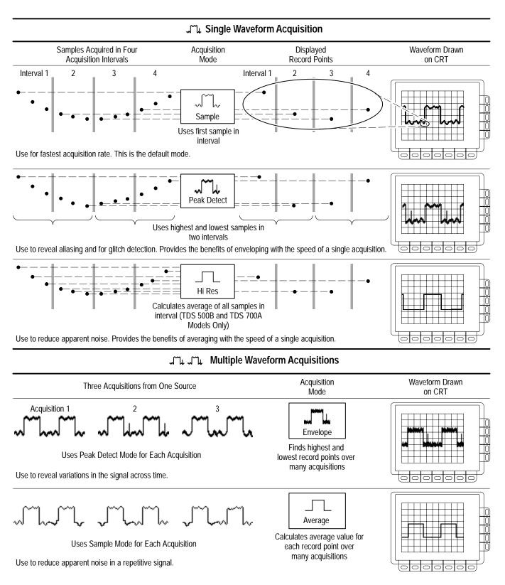
Figure 3–13: How the Acquisition Modes Work
