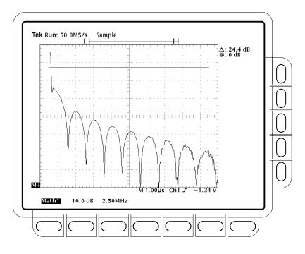
Figure 3–89: Cursor Measurement of an FFT Waveform
