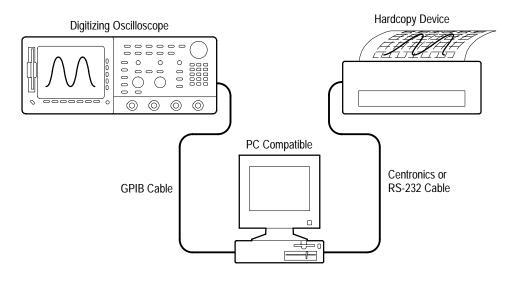
Figure 3–74: Connecting the Oscilloscope and Hardcopy Device Via a PC
