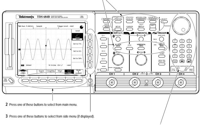
4 If side menu item has an adjustable value (shown in reverse video), adjust it with the general purpose knob or keypad.
