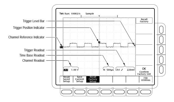
Figure 2–5: The Display After Factory Initialization
