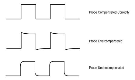
Figure 3–1: How Probe Compensation Affects Signals
