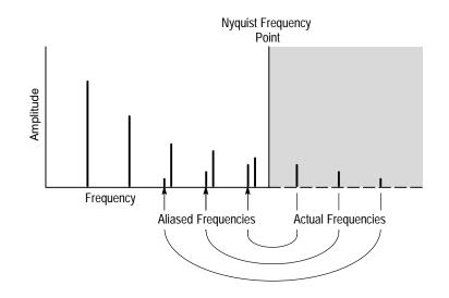
Figure 3–92: How Aliased Frequencies Appear in an FFT
