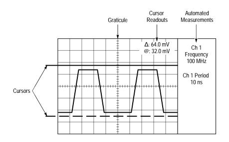
Figure 3–51: Graticule, Cursor and Automated Measurements
