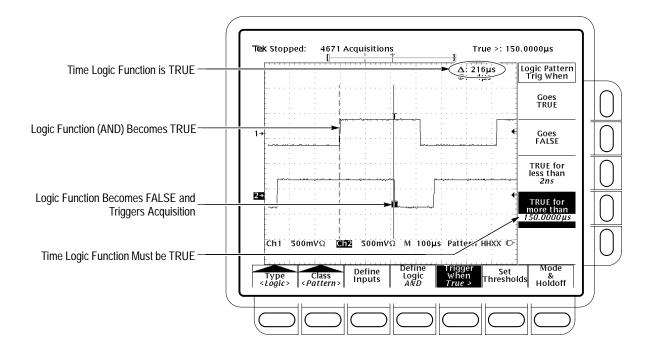
Figure 3–41: Logic Trigger Menu — Time Qualified TRUE
