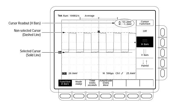
Figure 3–60: H Bars Cursor Menu and Readouts
