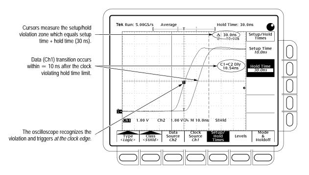
Figure 3–42: Triggering on a Setup/Hold Time Violation
