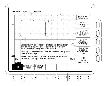
Figure 3–87: Define FFT Waveform Menu
