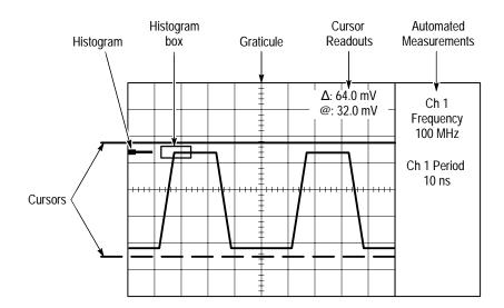
Figure 3–58: Histogram, Graticule, Cursor and Automated Measurements
