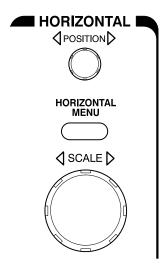
Figure 3–8: Horizontal Controls
