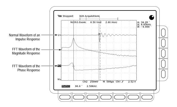
Figure 3-96: System Response to an Impulse
