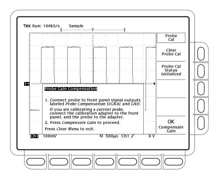
Figure 3–73: Probe Cal Menu and Gain Compensation Display
