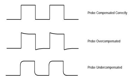
Figure 3–1: How Probe Compensation Affects Signals
