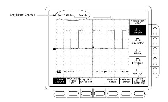
Figure 3-16: Acquisition Menu and Readout
