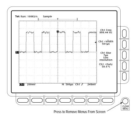
Figure 2–15: Four Simultaneous Measurement Readouts
