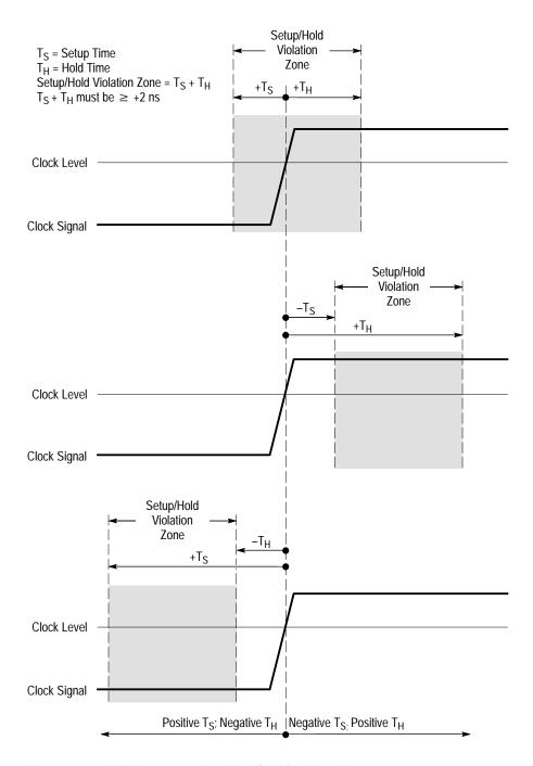
Figure 3-44: Violation Zones for Setup/Hold Triggering
