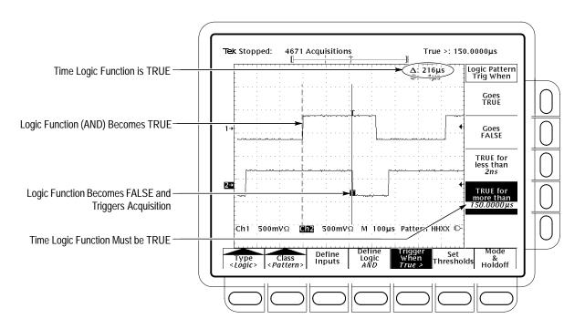
Figure 3–47: Logic Trigger Menu — Time Qualified TRUE
