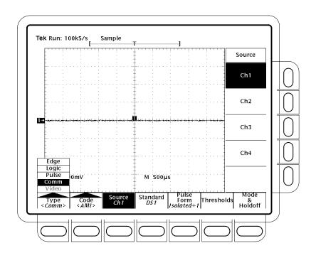
Figure 3–53: Main Trigger Menu — Comm Type
