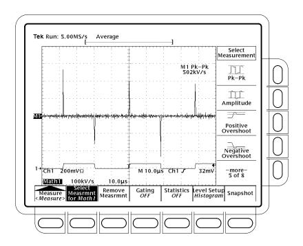
Figure 3–106: Peak-Peak Amplitude Measurement of a Derivative Waveform
