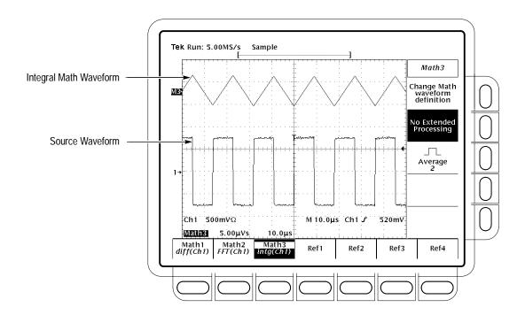
Figure 3-107: Integral Math Waveform
