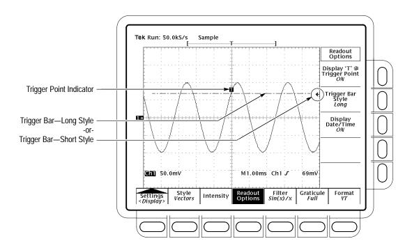
Figure 3-20: Trigger Point and Level Indicators
