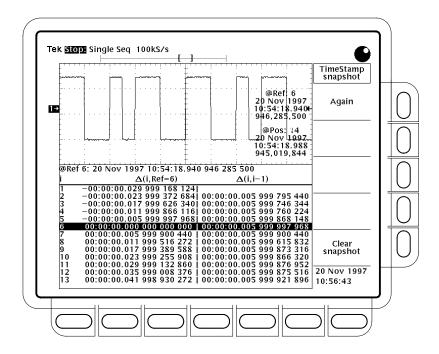
Figure 3–34: Horizontal Menu — FastFrame Snapshot
