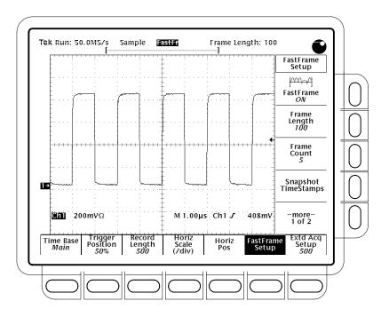
Figure 3-33: Horizontal Menu — FastFrame Setup
