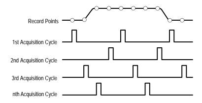
Figure 3–14: Equivalent-Time Sampling
