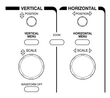
Figure 2-6: The VERTICAL and HORIZONTAL Controls
