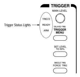
Figure 3–39: TRIGGER Controls and Status Lights
