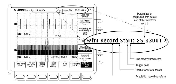
Figure 3-10: Extended Acquisition Length and Zoom
