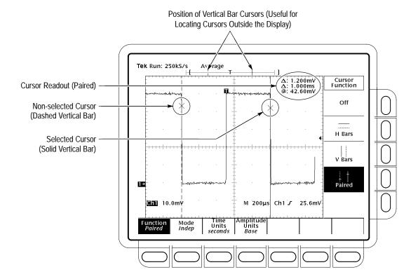
Figure 3-68: Paired Cursor Menu and Readouts
