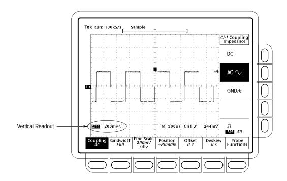
Figure 3-6: Vertical Readouts and Channel Menu
