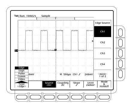
Figure 3–43: Main Trigger Menu — Edge Type
