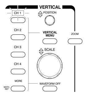
Figure 2–11: The Channel Buttons and Lights
