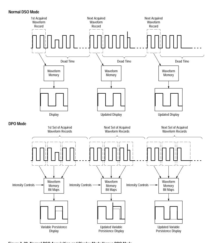
Figure 3–28: Normal DSO Acquisition and Display Mode Versus DPO Mode
