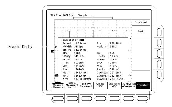
Figure 3-64: Snapshot Menu and Readout
