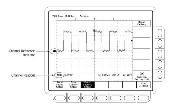
Figure 3-3: The Channel Readout
