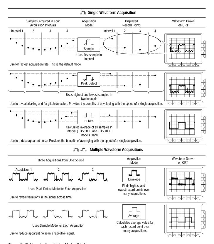
Figure 3–15: How the Acquisition Modes Work
