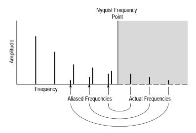
Figure 3–102: How Aliased Frequencies Appear in an FFT
