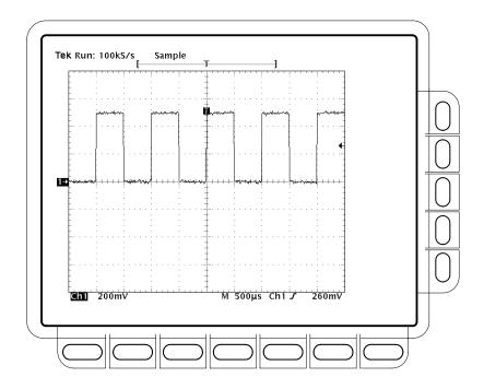
Figure 2–9: The Display After Pressing Autoset
