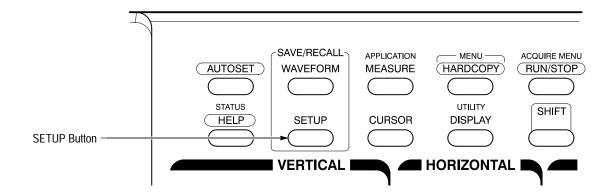
Figure 2–2: SETUP Button Location
