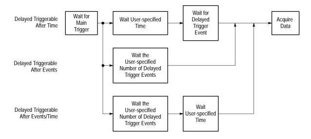
Figure 3-55: Delayed Triggerable
