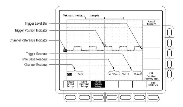
Figure 2–5: The Display After Factory Initialization
