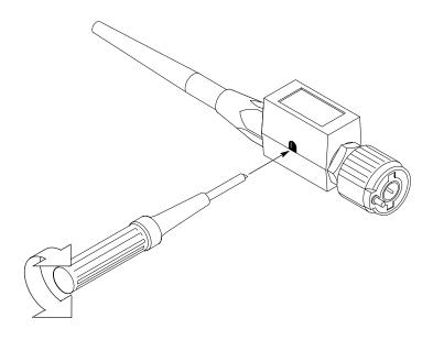
Figure 3-2: P6139A Probe Adjustment
