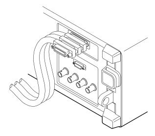
Figure 3-86: Stacking GPIB Connectors
