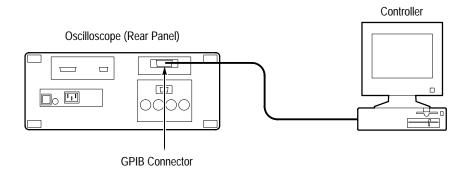
Figure 3–87: Connecting the Oscilloscope to a Controller
