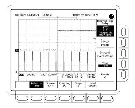
Figure 3-57: Delayed Trigger Menu
