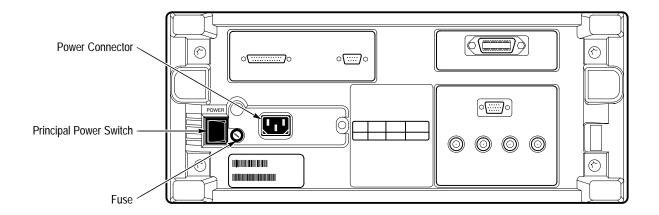
Figure 1–1: Rear Panel Controls Used in Start Up
