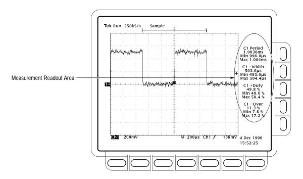
Figure 3-59: Measurement Readouts with Statistics
