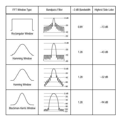
Figure 3-104: FFT Windows and Bandpass Characteristics
