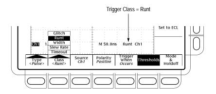
Figure 3-49: Pulse Trigger Readouts
