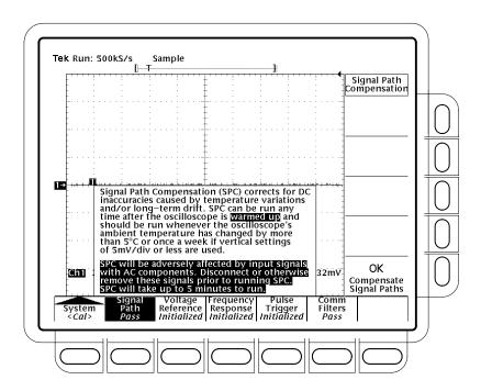
Figure 3–72: Performing a Signal Path Compensation
