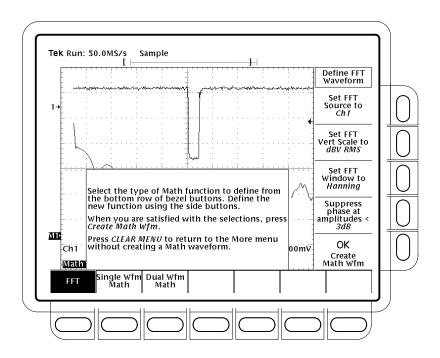
Figure 3-97: Define FFT Waveform Menu
