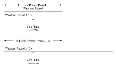
Figure 3-100: Waveform Record vs. FFT Time Domain Record
