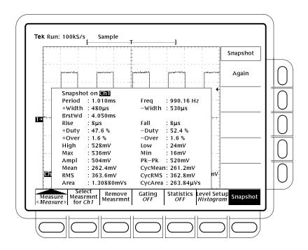
Figure 2-17: Snapshot of Channel 1
