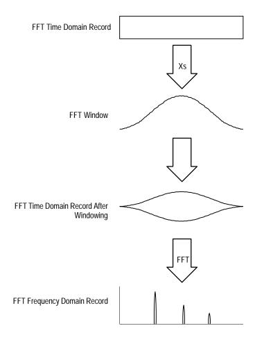
Figure 3-103: Windowing the FFT Time Domain Record
