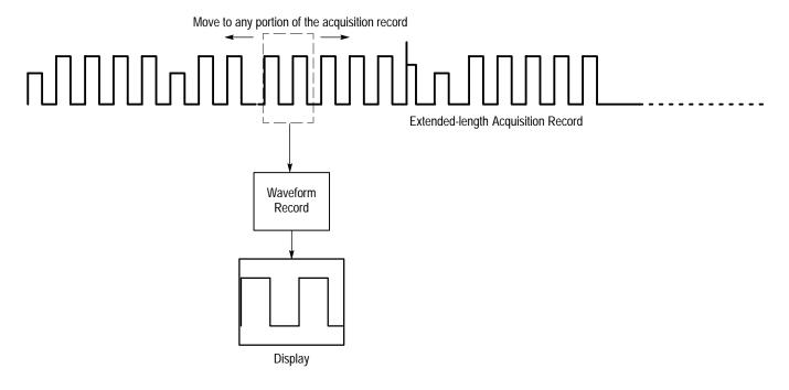
Figure 3-9: Displaying an Extended Acquisition Length Record
