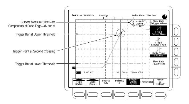
Figure 3-52: Main Trigger Menu — Slew Rate Class
