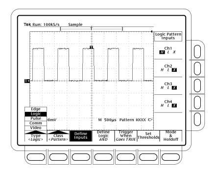
Figure 3-46: Logic Trigger Menu
