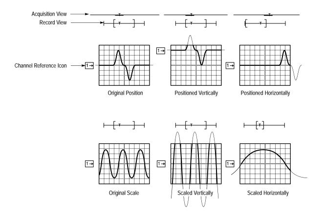
Figure 3–5: Scaling and Positioning
