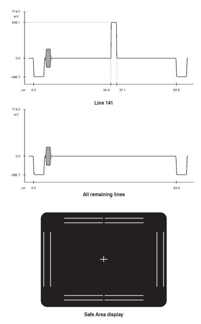
Figure 16 (cont.): Safe Area Signal Components
