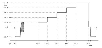
Figure 7: 5-Step Staircase (Gray Scale)
