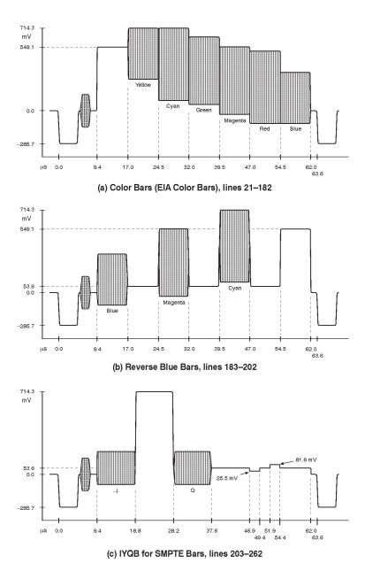
Figure 5: SMPTE Color Bar Signal Components
