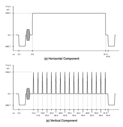
Figure 14: Convergence Signal Components
