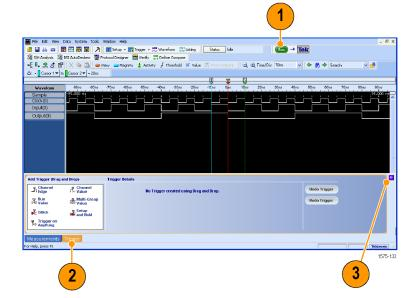
Click and drag the Channel Edge icon from the Tabbed Trigger window to the Output waveform.
