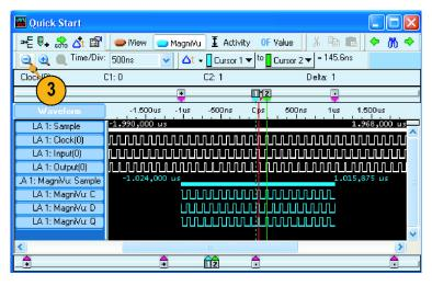
Move Cursor 1 to an area in the Waveform window outside the range of the MagniVu data.
