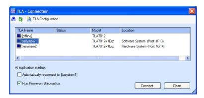
NOTE. To start the TLA Server on TLA7012 and TLA6400 instruments, right-click the (TLA Server) icon in the toolbar at the bottom right side of the screen and select **Start TLA Server**.
