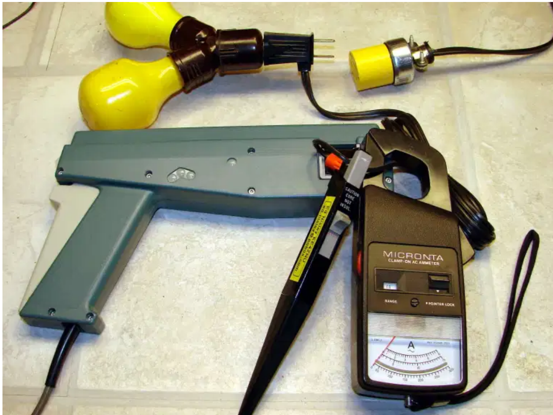
Tektronix A6302 A6303 Current Probes – test load
