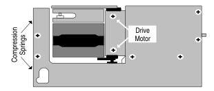
**7.** Remove the two mounting screws that hold the motor drive assembly to the right side panel. They are located near the middle of the right side panel.
