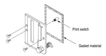
3. Inspect gasket material and replace if necessary (use Dow Corning 3140 or equivalent to coat mating surface of gasket).
