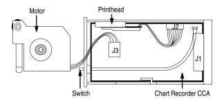
The illustration above shows the connector locations in the YT-1/YT-1S. Each connector and the signals that should be found on them are described in the following paragraphs and tables.
