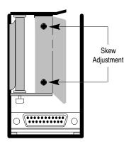
2. The two screws holding the paper guide onto the motor assembly must be loosened slightly (not too much!). Position the paper guide as follows:
