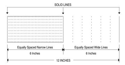
a. The total chart from first printed line to last printed line must measure between 10.87 to 12.76 inches.
