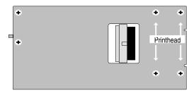
**11.** Carefully disconnect the thermal printhead from the ECB. Use an IC puller or a long-nosed plier.
