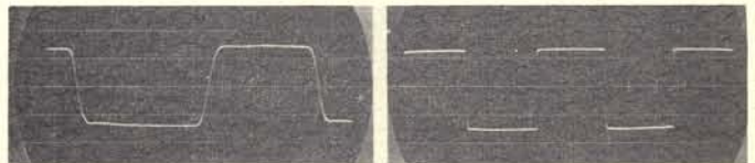
Fig. 1. 1 megacycle square wave. Fig. 2. 60 cycle square wave. Response of 2 Stage Vertical Amplifier.
