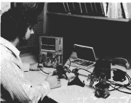
Millimeter wave test set-up using the 7L18 spectrum analyzer with external waveguide mixer.
