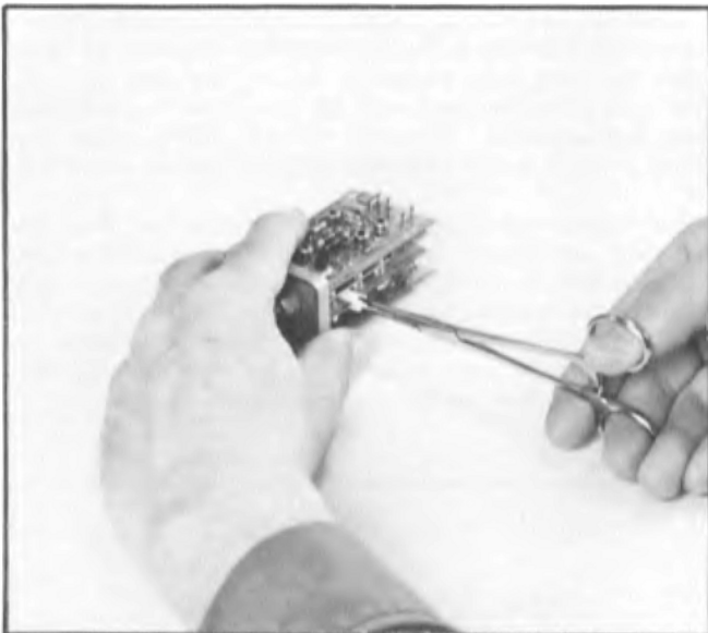
Fig. 4-2. Removal or replacement of sampling bridge diodes.
