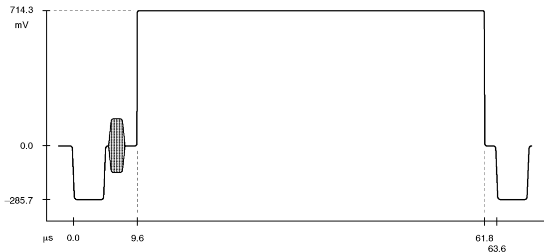
Figure 1-39: NTSC 100 IRE, Field Square Wave (and Bounce, High)
