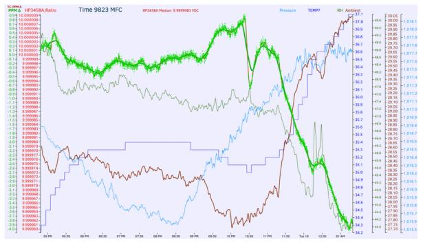
Tempco of the output voltage seem to be **-1.9ppm/°C** which is bit high, but actually fits specifications of  $\pm 2ppm/°C$ . We will be checking later if it's possible to improve stability and reduce temperature sensitivity. For comparison, industry standard multifunction calibrators, such as Fluke 5700A offering  $\pm 0.24ppm/°C$  at 10VDC, in 10°C to 40°C window (22VDC specification  $\pm 0.2ppm/°C + 0.4\mu$ V).
