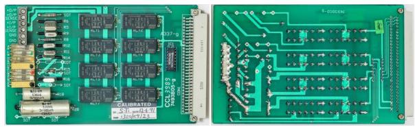
This assembly is resistance standard of calibrator. Even without schematics it's operation is very easy to understand. **SN7445N** BCD-to-DECIMAL decoder switches on one of eight **S4-12V relays**, which are connecting one of reference resistors to 4-wire Kelvin output at CON2 terminal block or bypass these resistors for voltage/current output.
