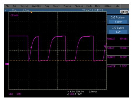
I tried replacing old optocouplers with brand new Vishay ILD74's but that help nothing, calibrator still had same issues with voltage output being adjusted in large steps only from MSB discrete DAC ladder.
