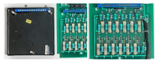
D/A PCB have array of 12 ultra-precision **3ppm/°C AX175/C wire-wound resistors** paired with good quality trimmers. Perhaps this is to allow linearity adjustment, if DAC used have 12-bit resolution?
