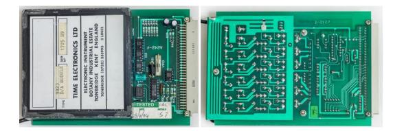
Similar to reference, D/A converter is potted in black epoxy box, marked **9823 D/A MODULE** with serial code **1725 H9**, whatever that means. It's hard plastic, so there is little chance of taking it apart without damaging circuits inside.
