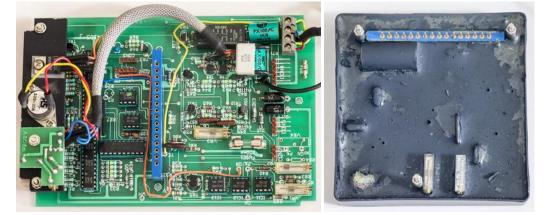
Potted reference-amplifier module accepts ±18V input power supply from backplane connector and provides stable voltage or current reference for rest of the calibrator.
