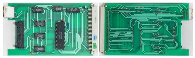
GPIB interface controller is rather simple board, with MC68488 GPIB interface controller for M6800 Motorola MPU processor family and four more MC3448A GPIB transceivers. Couple more 74-series logic packages doing some minor glue function.
