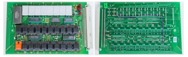
LED 7-segment display is controlled by Intersil ICM7218, which is 8-digit LED microprocessor-compatible multiplexed display decoder driver. It's 5V logic chip, capable of driving segments at 40mA, with 250Hz scan rate.
