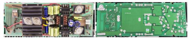
This board generates an unregulated voltage approximately  $\pm 4V$  to supply high-current source. This voltage is regulated by push-pull stage to provide up to 10Amps of current.
