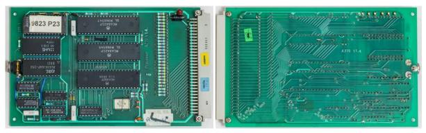
This is where digital brain of the instrument reside. Good old friend, **Motorola MC6802 8-bit processor** is in charge. It does have internal 1MHz clock oscillator and 128 bytes of RAM and have 16-bit memory address bus. Two **Motorola MC6821 Peripheral Interface Adapter** chips provide GPIO function for the rest of the instrument, with 32 I/O signals on each IC.
