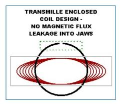
Wrap Round Coil Design where jaw opening is inside the coils field gives potential for magnetic flux leakage increasing reading errors.
