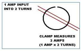
It is this principle, which enables a clamp meter to be calibrated at much higher currents than is directly available. By producing a coil with a known number of turns the input current is multiplies by the number of turns on the coil.
