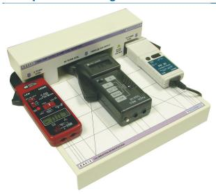
When a current is passed through a wire, a magnetic field, which is proportional to the current, is created around the wire.
