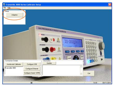
To configure the adapter, first connect the adapter to the Adapter Interface connection on the front of the calibrator. If the adapter is fitted with a power LED this will light up to indicate correct connection.
