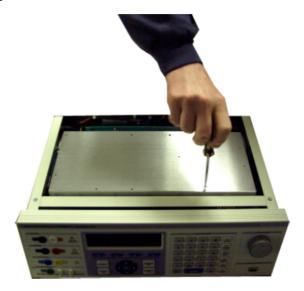
Remove the top screening cover of the PCB – remove all nylon fixing screws, plus 1 metal screw from far end of PCB cover.
