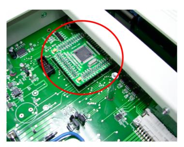
6. After fitting the replacement processor re-assemble the unit by repeating steps 1-4 in reverse, ensuring that all screws are tight.
