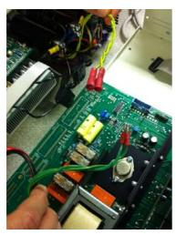
SEPARATE BULLET CONNECTIONS FROM REAR PANEL LEADS
