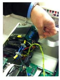
REMOVE CONNECTOR FROM TOP OF TRANSFORMER PCB
