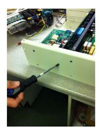
REMOVE SIDE FIXING SCREWS WHICH HOLD THE MIDDLE BOARD IN PLACE
