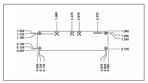
The base mounting screw holes (4) accommodates  $\#6/32 \ge 3/8$  machine screws. When mounting the Mini-T onto a plate for permanent mounting, take into consideration the length of the screw and the thickness of the plate so that the screws do not protrude into the Mini-T and potentially damage electronics.
